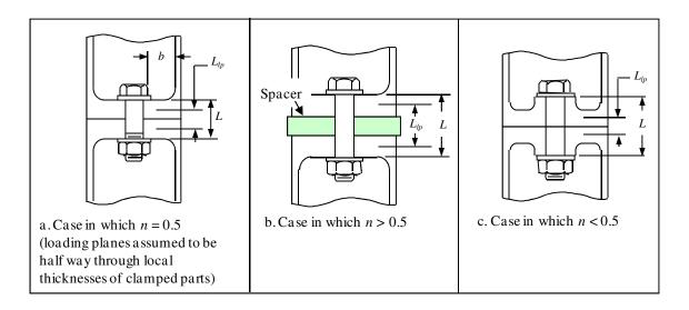
Figure 4—Dimensions Used to Calculate Load-Introduction Factor
