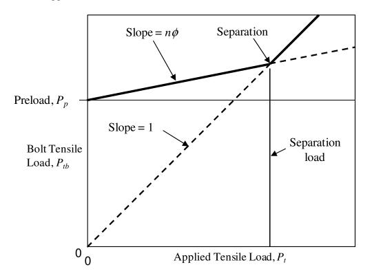
Figure 10—Bolt Tensile Load versus Applied Tensile Load
