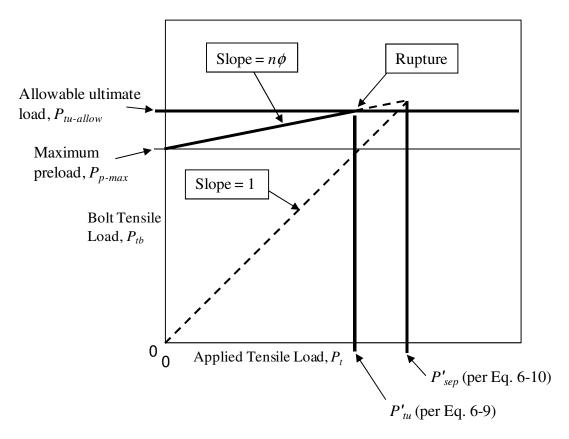
**Figure 12—Rupture Before Separation with Linear Theory**
