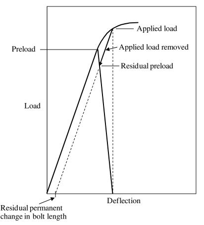
Figure 16—Loss of Preload Resulting from Fastener Yielding
