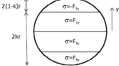
Figure 13—Stress Distribution at Collapse Due to Combined Bending and Tension
