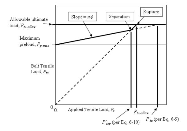
**Figure 11—Separation Before Rupture with Linear Theory**
