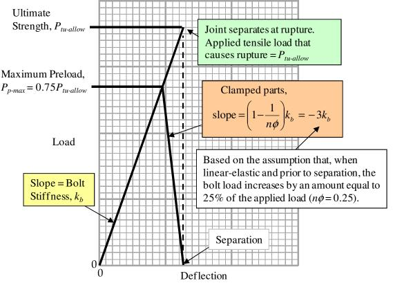
Figure 8—Separation Before Rupture for a Brittle Threaded Fastening System
