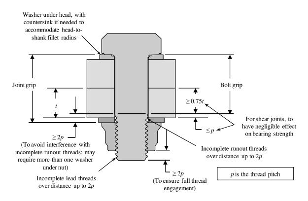
**Figure 2—Dimensional Considerations in Selecting Fastening Hardware**
