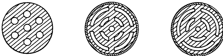
Figure 25.—Typical multiperforated grain shapes.
