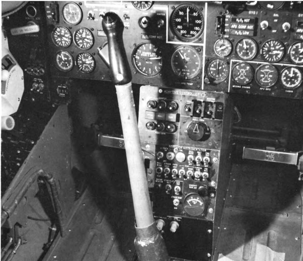
This is the centrally placed control panel of the X-15's remarkable and highly successful adaptive-control system.
