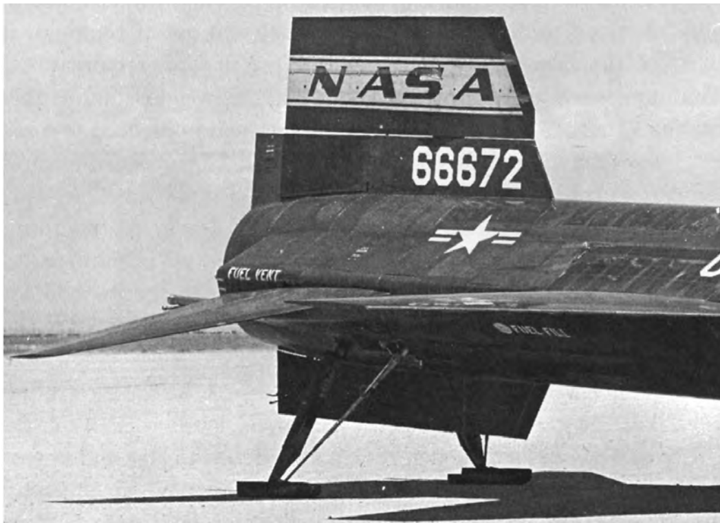
This photograph provides an unusually clear view of the X-15's unique main landing gear, and shows how much of the lower vertical tail is left after its bottom part has been jettisoned for landing. The photo also reveals the new, knife-sharp leading edge that has been given to the X-15-3 configuration's upper vertical tail in order to study heat transfer through 2500-deg. airflow.
