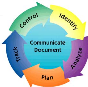
Figure 2-2: The Continuous Risk Management Process
