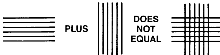
FIGURE 16. FATAL FLAW IN TENSOR-POLYNOMIAL COMPOSITE FAILURE CRITERIA
