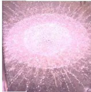
Figure 4.6-7. Rear wall after impact.
