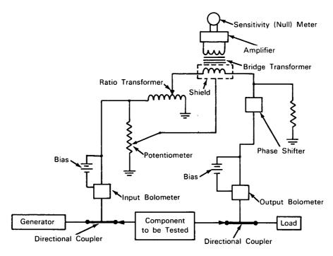
The problem: Accurate measurement of the insertion loss of rf components while avoiding the effects of amplifier drift.
