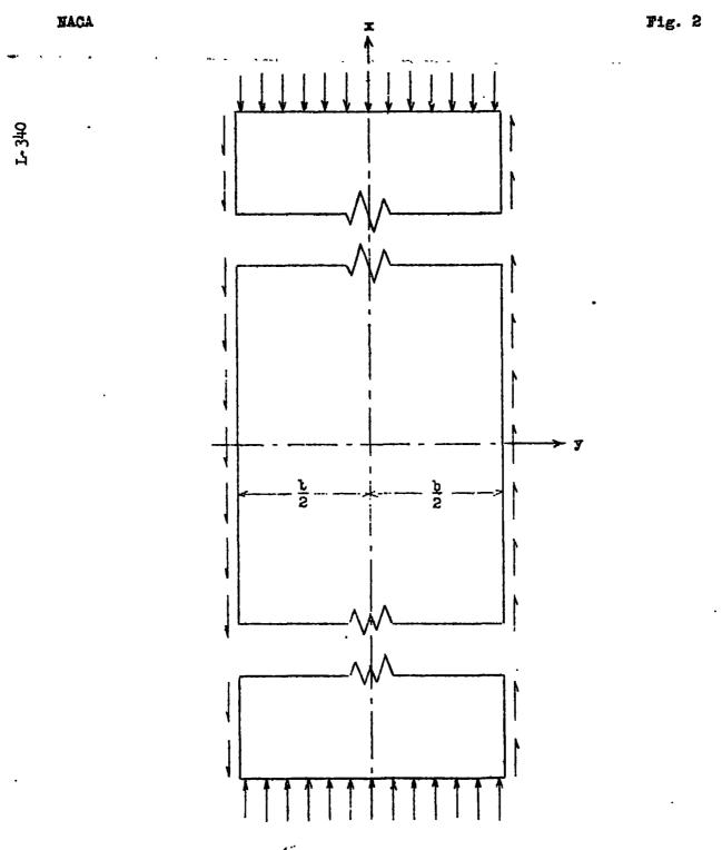
Figure 2.- Infinitýly long rectangular plate under combined shear and compression; coordinate system used in appendix A.
