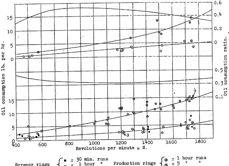
Scraper rings  $\begin{cases} \bullet = 30 \text{ min. runs} \\ \circ = 1 \text{ hour } \text{"} \\ \circ = 1 \text{ hour } \text{"} \end{cases}$  Production rings  $\begin{cases} \bullet = 1 \text{ hour runs} \\ \bullet = 5 \text{"} \end{cases}$  Oil consumption ratio =  $\frac{\text{Scraper ring oil consumption}}{\text{Production ring oil consumption}}$
