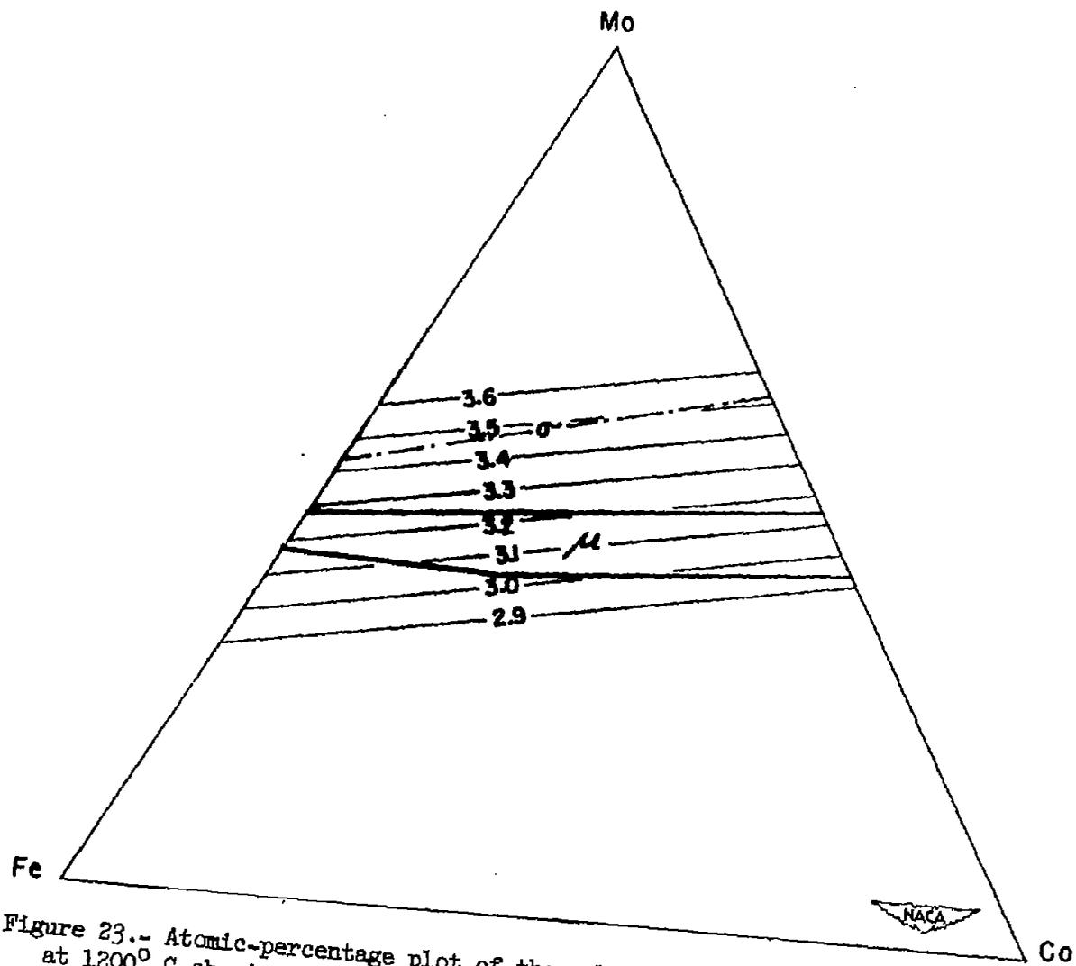
Figure 23.- Atomic-percentage plot of the cobalt-iron-molybdenum ternary system at 1200° C showing location of intermediate phases in relation to electron equivacancy lines.
