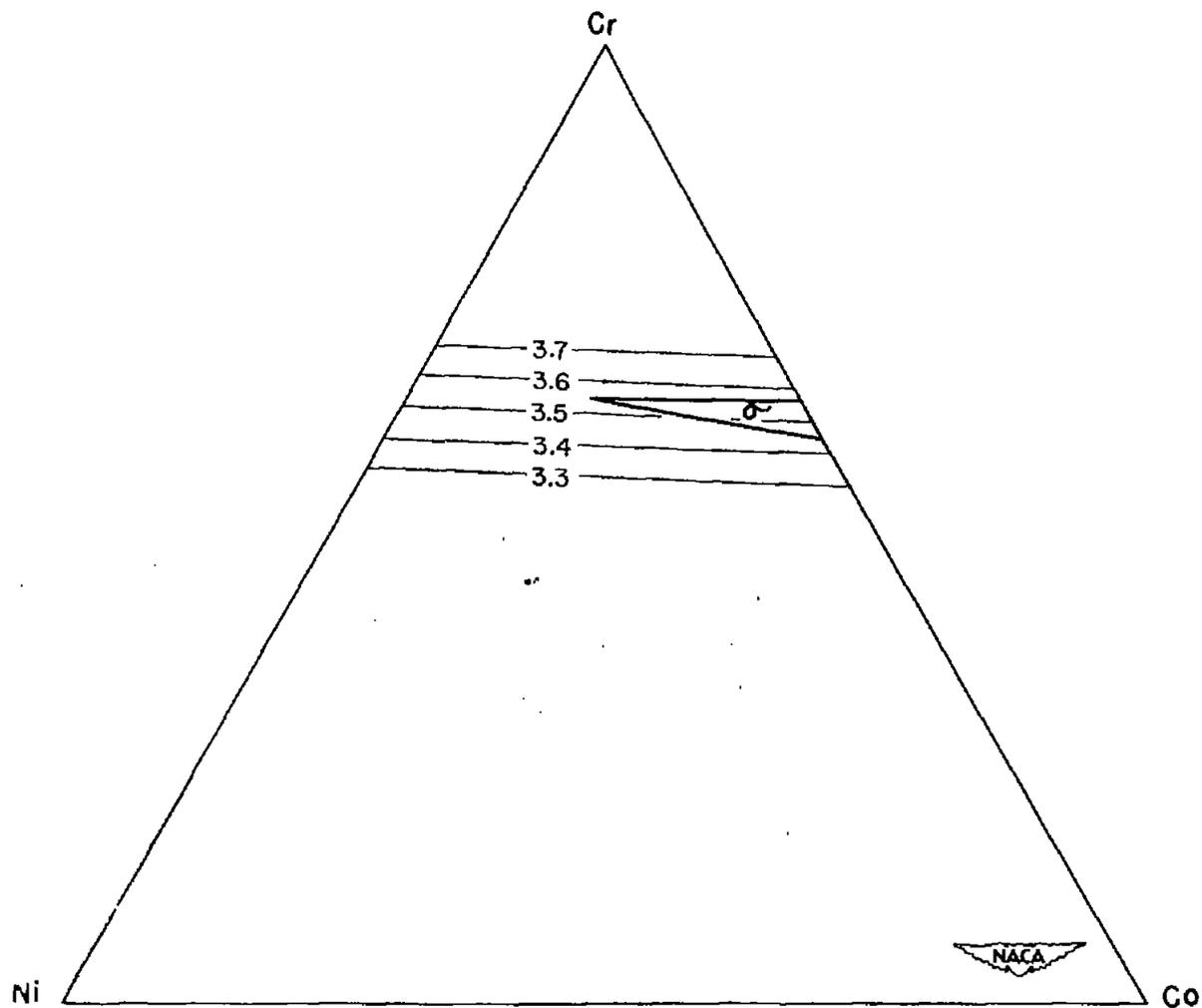
Figure 26.- Atomic-percentage plot of the cobalt-nickel-chromium ternary system at 1200° C showing location of intermediate phases in relation to electron equivacancy lines.
