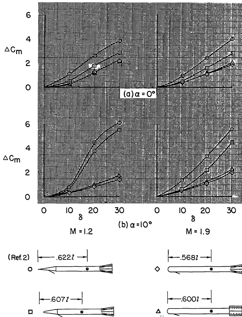
Figure 11.- Control effectiveness for the tail-on configurations.
