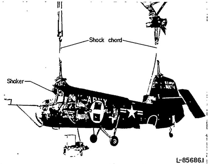
FIGURE I-4.—Test helicopter, with blade assemblies removed, showing method of suspension used for the ground vibration measurements.
