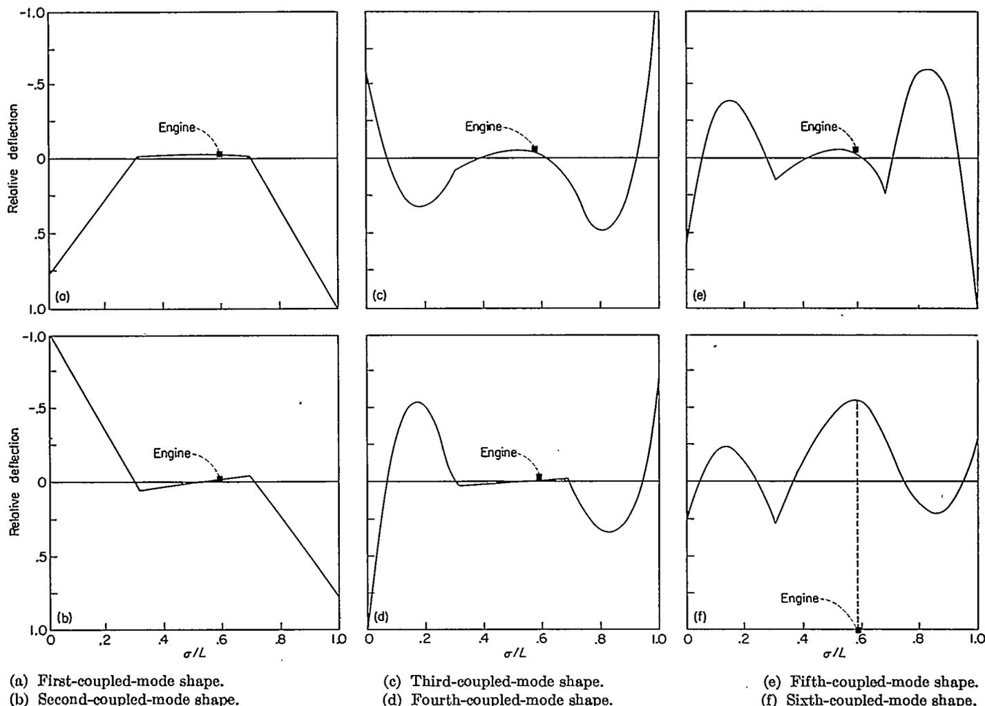
FIGURE II-3.—Mode shapes of coupled rotor-fuselage system.
