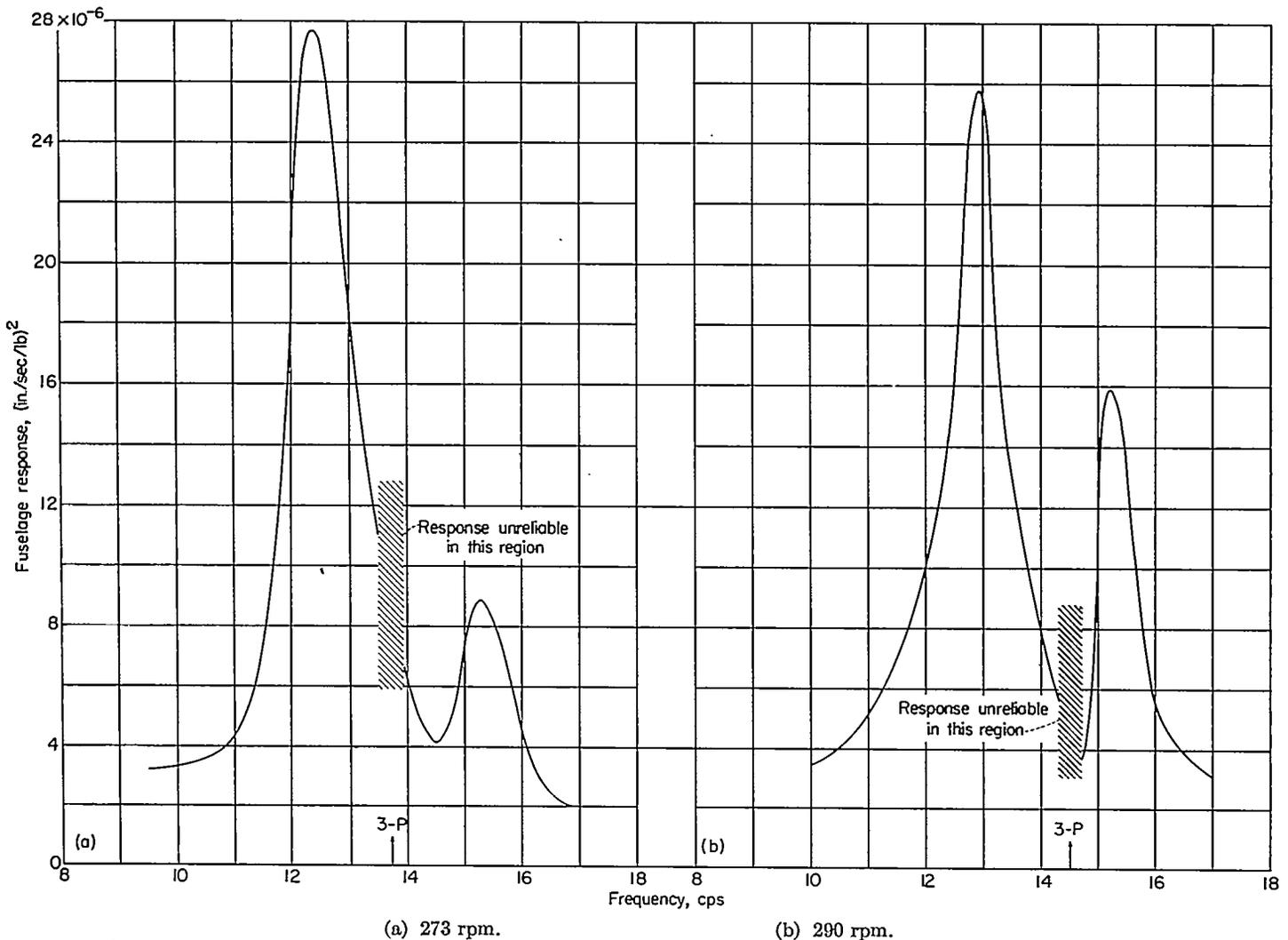
FIGURE I-8.—Coupled response of helicopter structure, measured at the front rotor, showing the effect of change in rotor speed for the wood blade configuration at a forward speed of 55 knots.
