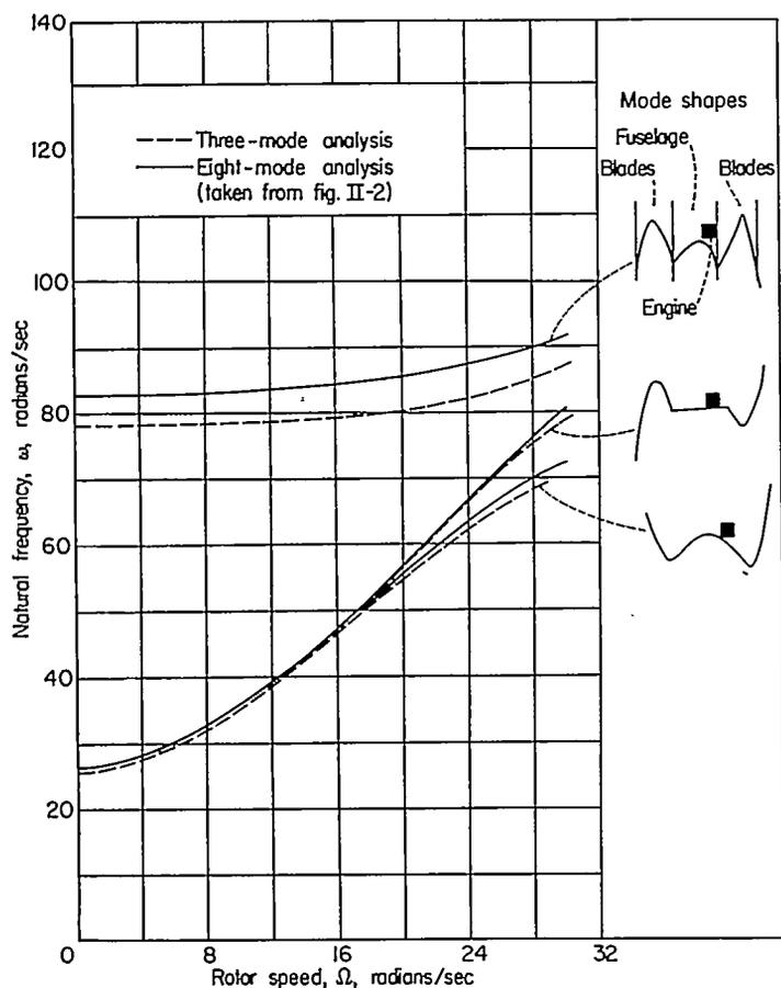
FIGURE II-6.—Comparison of natural frequencies of coupled system from three-mode analysis with corresponding frequencies from eight-mode analysis.
