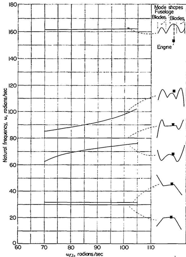
FIGURE II-4.—Effect of natural uncoupled frequency of fuselage on natural frequencies of coupled system.  $\Omega=30$  radians per second.
