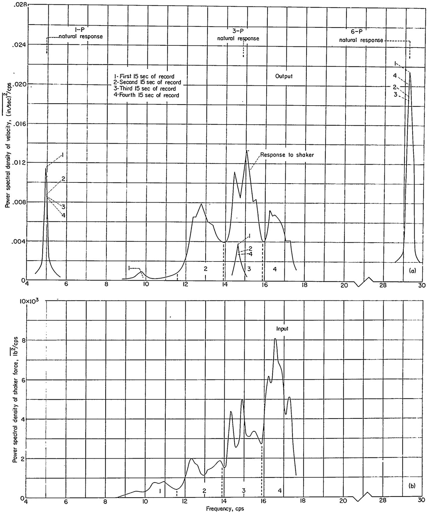
(a) Power spectrum of velocity at the front rotor.
