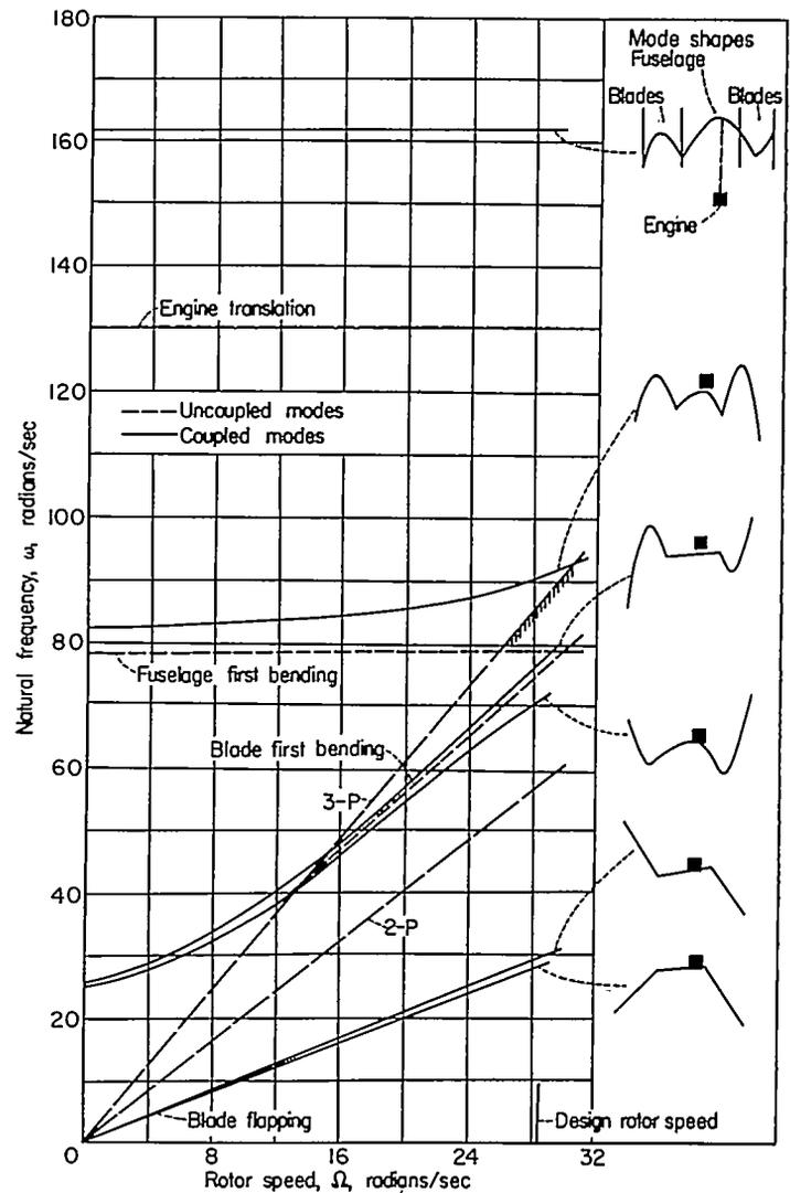
FIGURE II-2.—Variation of natural frequencies with rotor speed.
