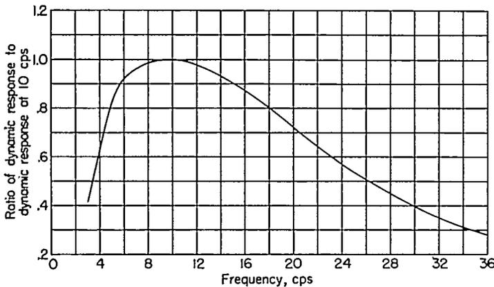
FIGURE I-3.—Typical response curve for vibration-pickup—oscillograph combination used.
