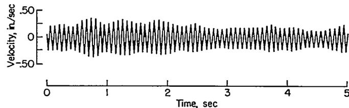
FIGURE I-12.—Sample record, showing the time variation of the 3-P component.
