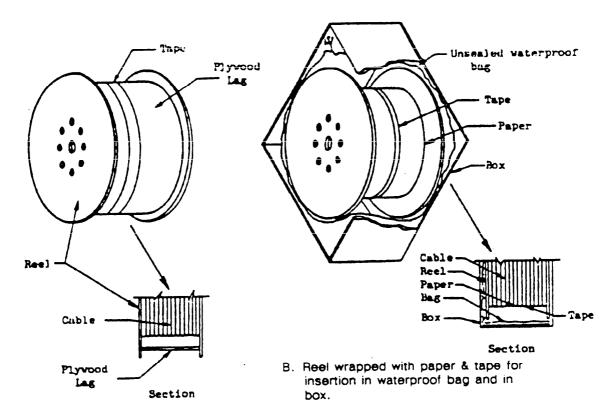
A. Reel enclosed with flexible plywood lagging. NOTE: The plywood lagging may optionally cover the outer edge of the reel.
