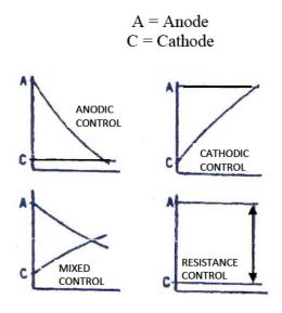
FIGURE B-1. Types of polarization and control in galvanic corrosion.
