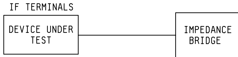
FIGURE 4116-2. Impedance bridge method .
