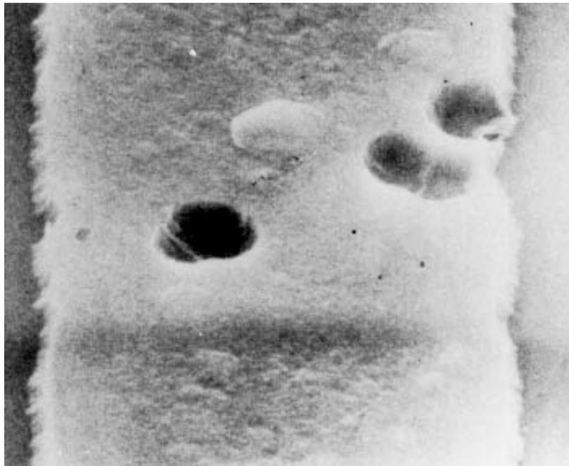
FIGURE 2077-18. (5,000X) General metallization voids (reject).
