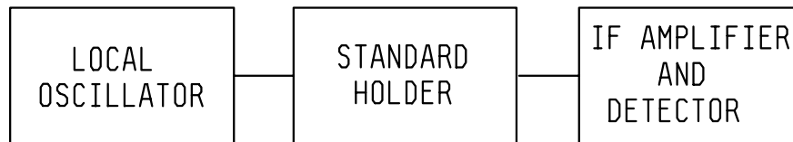
FIGURE 4121-1. Direct measurement method.
