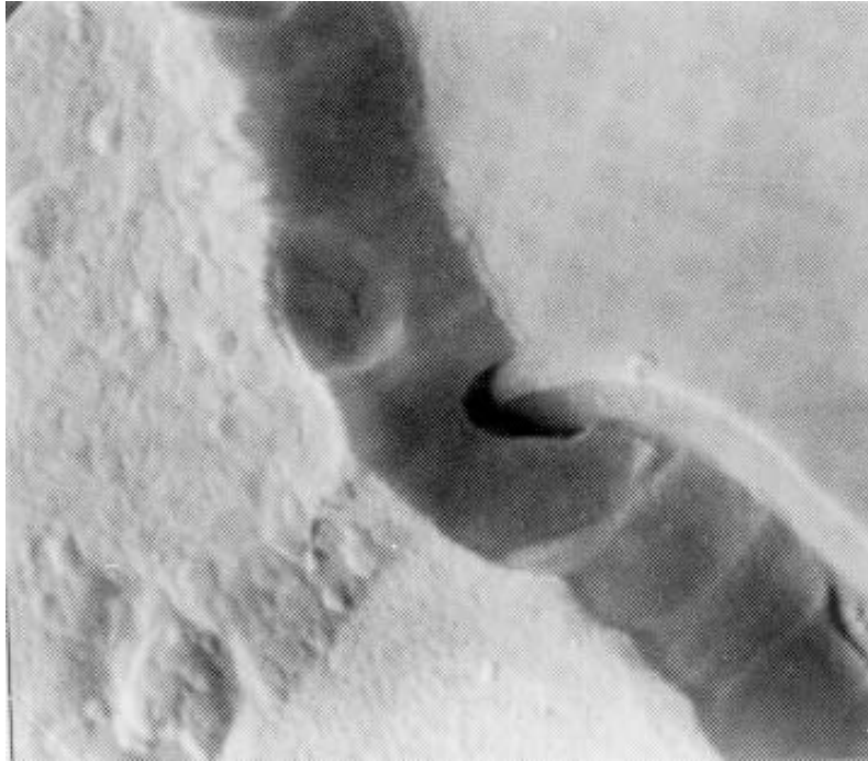
FIGURE 2077-8. Tunnel/cave at oxide step at 10,000X (accept).
