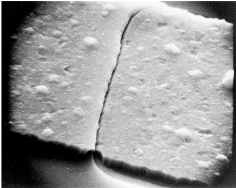
FIGURE 2077-9. Tunnel/cave at oxide step at 5,000X (reject).
