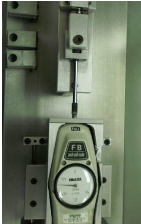
FIGURE 2038-1. Sample apparatus fixture with force measuring gauge.
