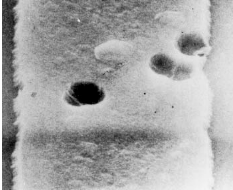
FIGURE 2077-20. General metallization voids at 5,000X (reject).
