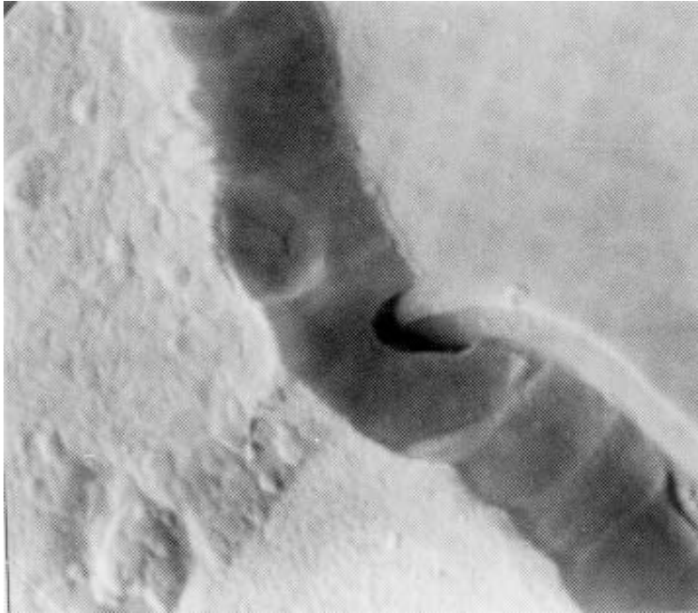
FIGURE 2077-8. Tunnel/cave at oxide step at 10,000X (accept).
