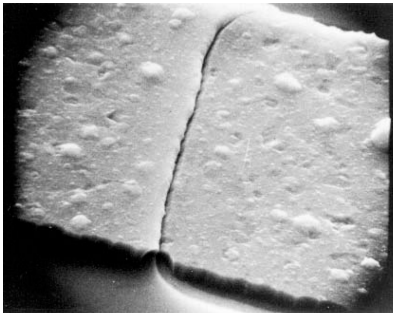
FIGURE 2077-9. Tunnel/cave at oxide step at 5,000X (reject).
