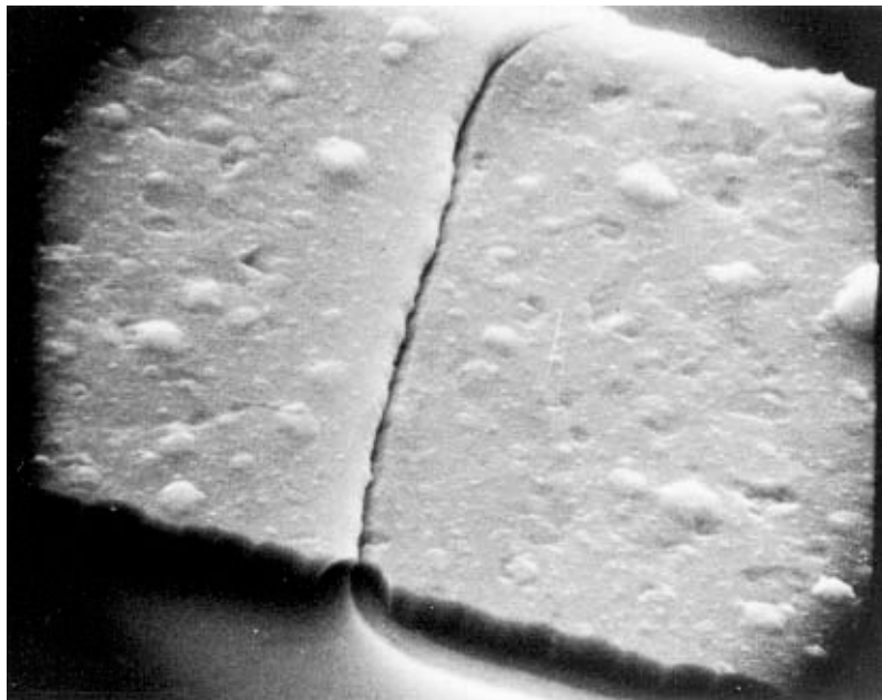
FIGURE 2077-9. Tunnel/cave at oxide step at 5,000X (reject).
