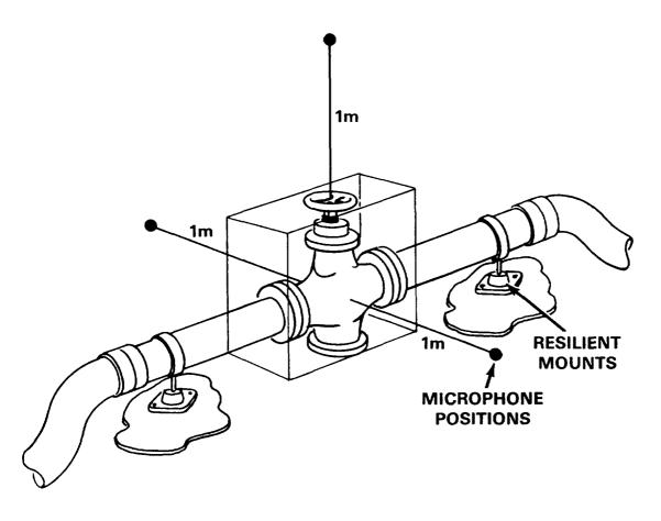
FIGURE 4. Sound measurement locations for valves.
