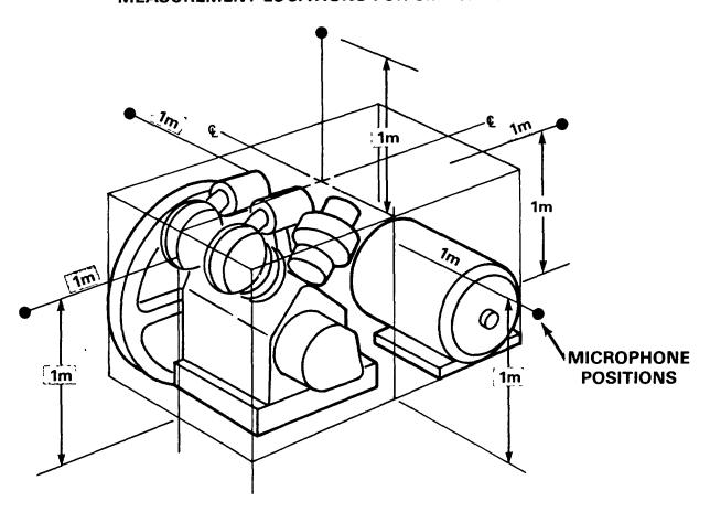
FIGURE 1. Sound measurement locations for small equipment,
