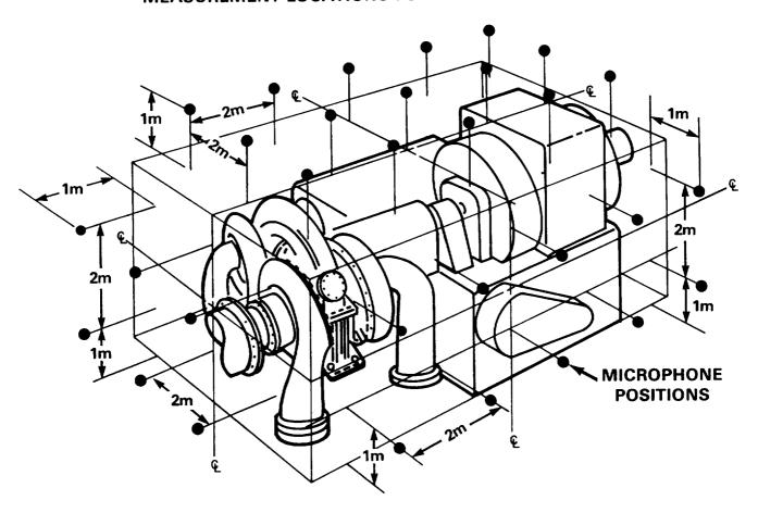
FIGURE 3. Sound measurement locations for large equipment.
