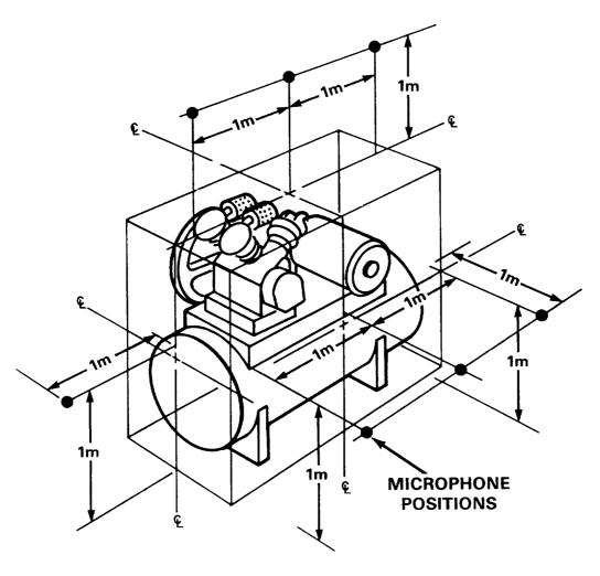
FIGURE 2. Sound measurement locations for medium size equipment, in addition to location of operator's head.
