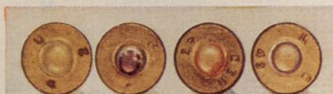
No. 37. No Waterproofing (Primer pocket joint)
