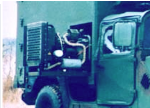
10 kW APU ready to slide into shelter.
