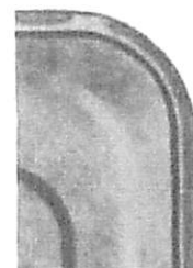
5-F. Lining Compound Containing Skips Less Than One Inch in Length— Minor
