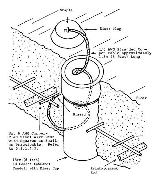
Figure 5. Typical Equipotential Ground Plane for Higher Frequency Facilities Installation (New Construction)
