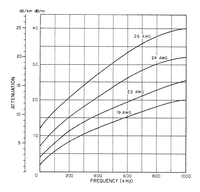
FIGURE 1. Attenuation versus frequency; AWG 19, 22, 24, 26
