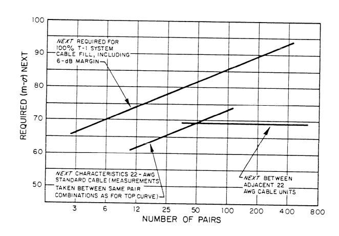
FIGURE 2. Near-end crosstalk characteristics.
