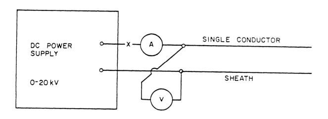
FIGURE C-4. Dieletric voltage withstand, conductor-to-sheath, symmetrical-pair or coaxial cable.
