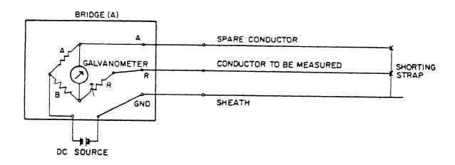
FIGURE C-1. First measurement of conductor resistance, Varley loop method.
