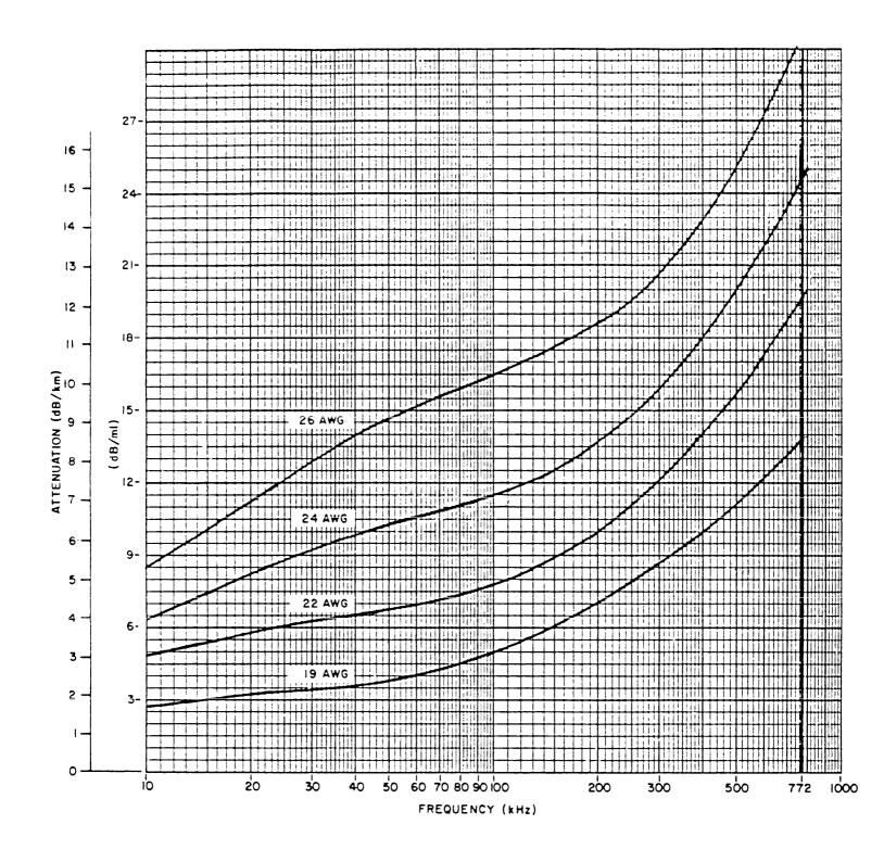
FIGURE 3. Carrier frequency attenuation.
