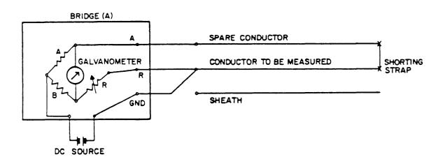
FIGURE C-2. Second measurement of conductor resistance, Varley loop method.
