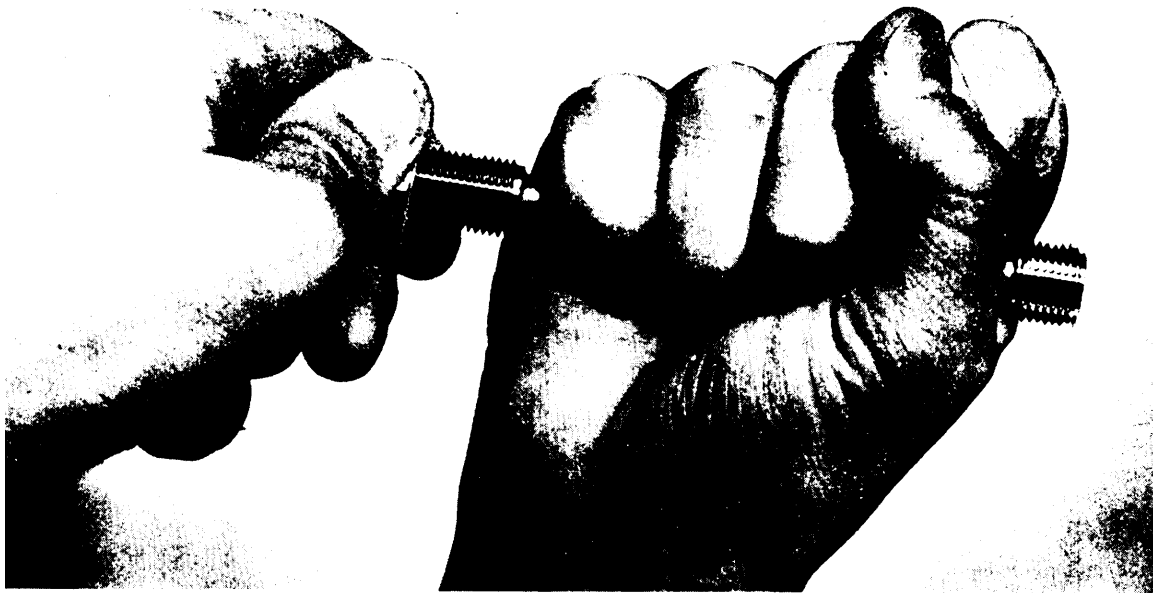
Figure 93. Improper method of inserting "Go" and "Not Go" thread plug gage.
