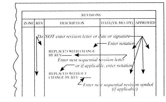
FIGURE 600–5. <u>Superseded (old) drawing notations redrawn with same</u> number
