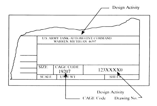
Figure 400-1. <u>Example of CAGE Code, drawing no, design</u> activity relationship as orginally specified.
