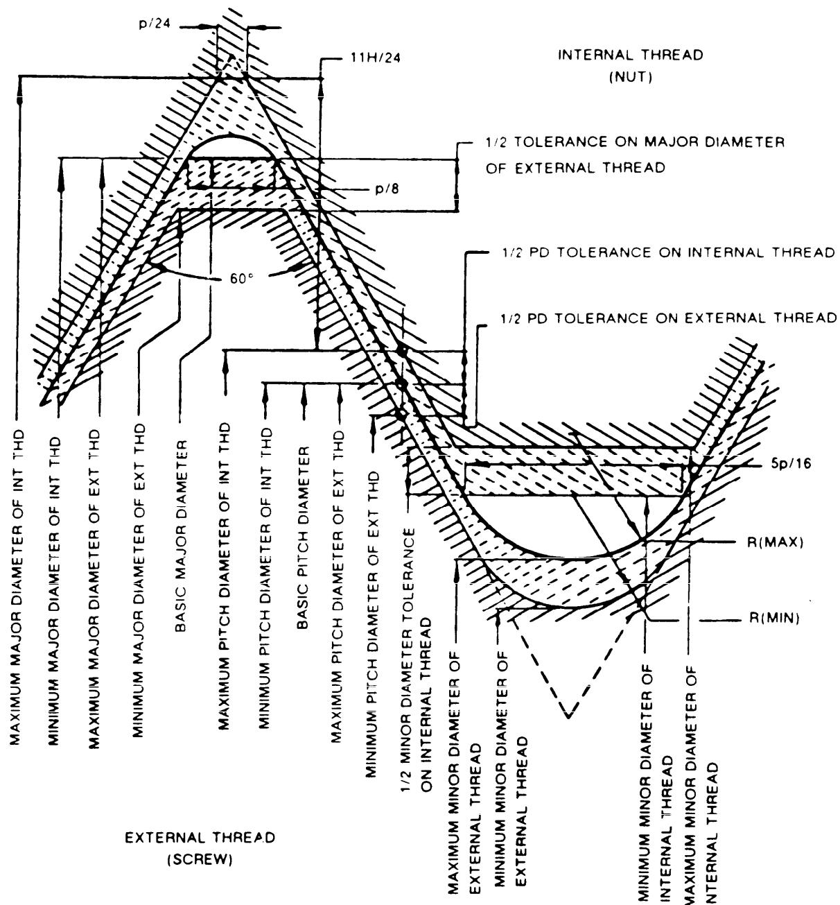
FIGURE 4. Disposition of tolerances and crest clearances.
