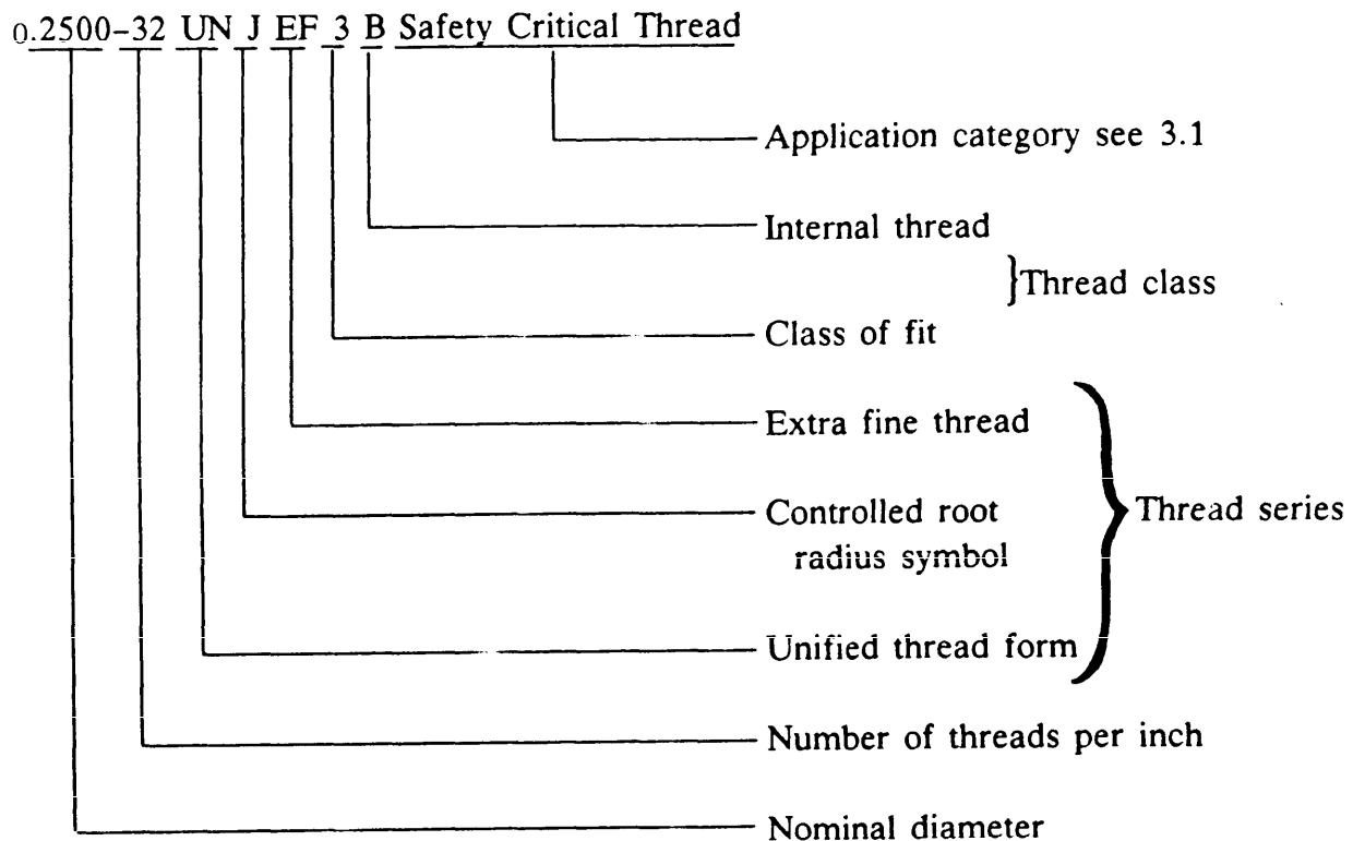
3.3.2 Special UNJ thread designations. The identifying letter "S" shall be included in the thread series symbol to indicate a special thread. Special diameter-pitch combinations developed in accordance with this specification shall be designated in the following manner:
