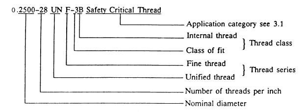
3.3.2 <u>Miniature thread designation</u>. The identifying letter "M" shall be included in the thread series symbol to indicate a miniature thread (see FED-STD-H28/5). Screw threads of this series shall be designated by their nominal diameters in millimeters followed by "UNM", the inch equivalent of the basic major diameter in parentheses which is optional, the number of threads per inch, class of thread, and external or internal threads.
