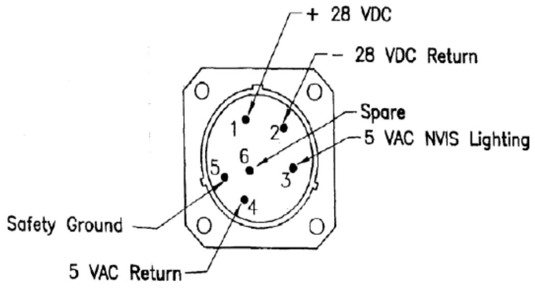
FIGURE 2. Wiring.
