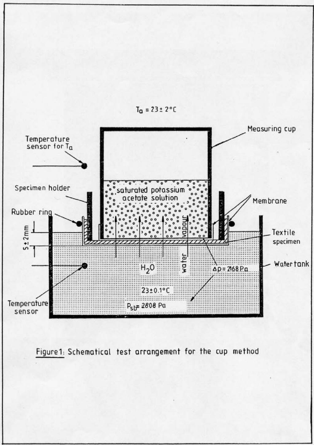
Figure1: Schematical test arrangement for the cup method
