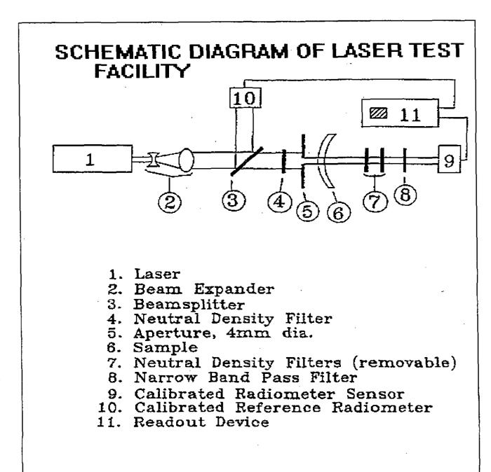
FIGURE 1. SPECTACLES, PROTECTIVE, LASER, BALLISTICS (BLIPS) SCHEMATIC DIAGRAM OF LASER TEST FACILITY
