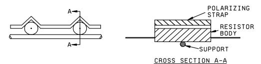
FIGURE 2. Mounting straps for moisture-resistance test.
