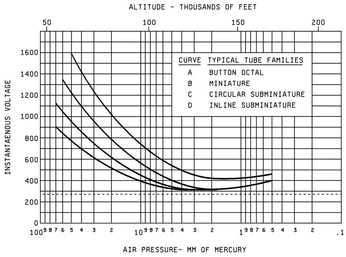
FIGURE 1. Reduced pressure (altitude) voltage breakdown characteristics.
