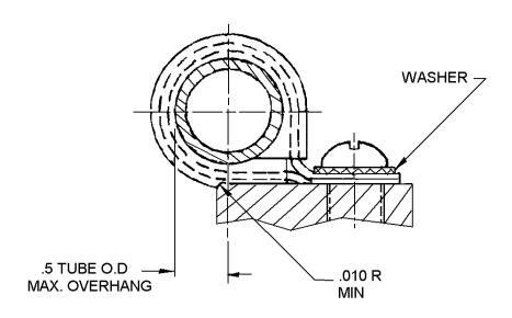
FIGURE 5. Recommended mounting of clamp at low to high vibration areas.
