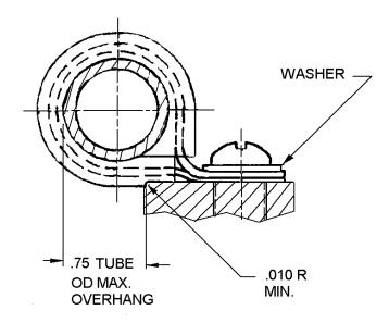
FIGURE 4. Recommended mounting of clamp at low to medium vibration areas.
