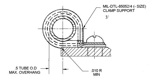
1/1 If MIL-DTL-85052/4 clamp supports are used, the maximum tube overhang shall be 0.5 tube. This clamp support can be detrimental if the clamp is not fully supported.
