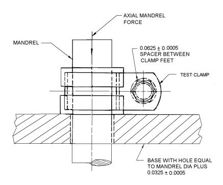
FIGURE 3. Clamp set up for diametral retention test.
