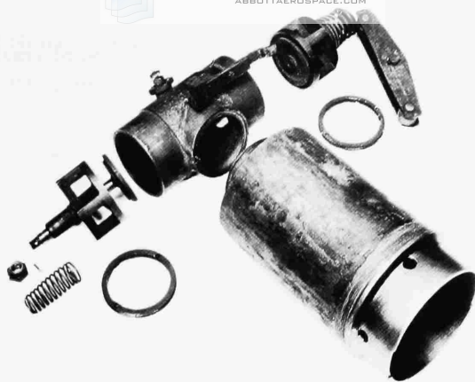
Figure 7.—First flight engine, 1903: cylinder, valve box, and gear mechanism; below, miscellaneous parts. (Photos courtesy Science Museum, London, and Louis P. Christman.)
