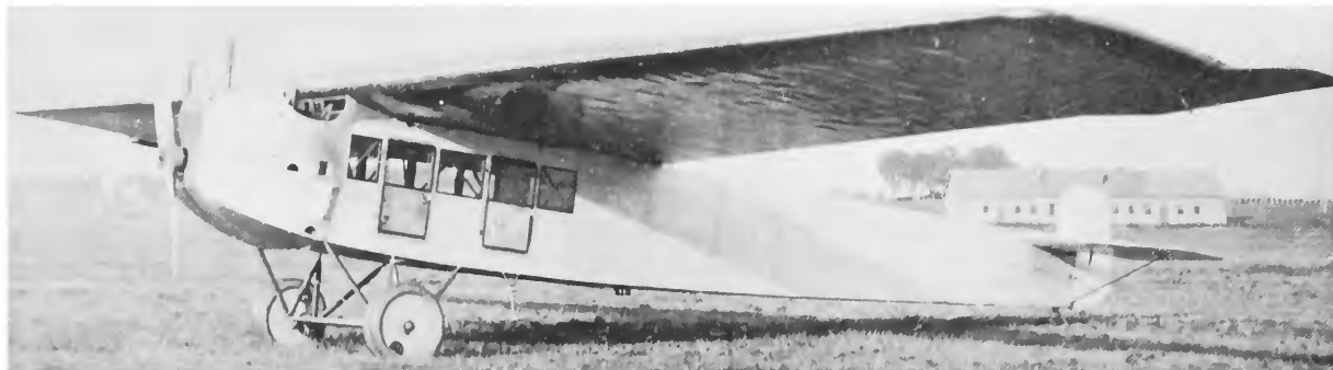
Figure 18.—Fokker F-IV showing original configuration.
