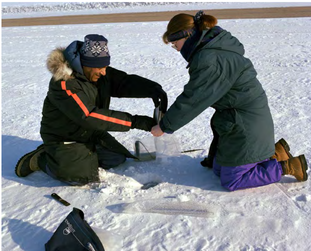
Figure 3-8. Joint Winter Runway Friction Measurement program, North Bay, Ontario, Canada. Researchers took manual measurements of ambient runway conditions before and after a test run series (NASA-LaRC photo EL-2000-00311).
