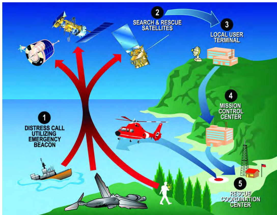
Figure 2-29. Search-and-rescue system (GSFC).
