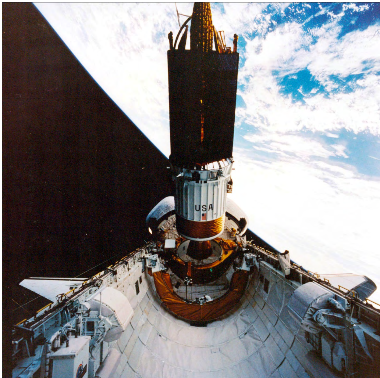
Figure 4-10. This photo shows TDRS-F as it is about to be released from its cradle/tilt table in Endeavour's cargo bay (NASA photo STS 054-71-025).
