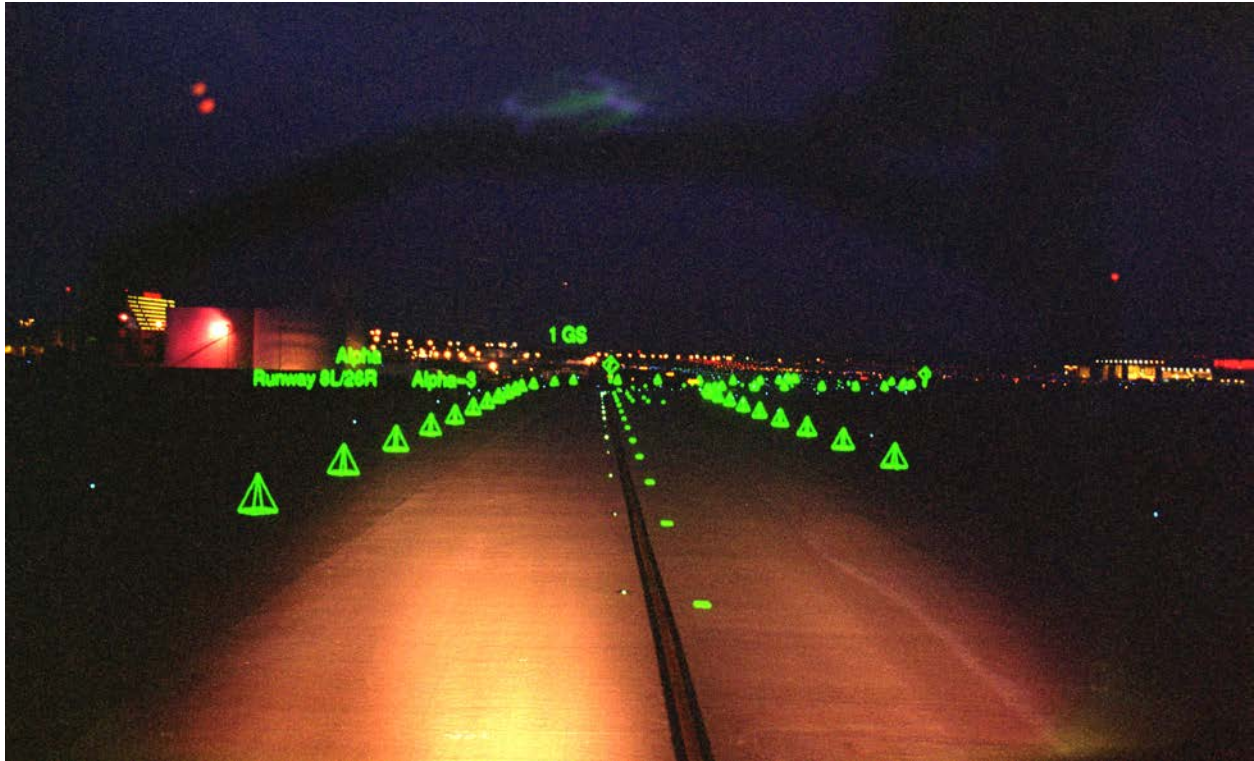
Figure 3-12. This photograph was taken from the cockpit window of NASA's 757 research aircraft during flight demonstration of airport capacity and safety enhancement technologies at Hartsfield-Atlanta International Airport in August 1997. As the 757 approached the runway, computer-generated graphics outlined the correct runway and its precise location on a "head-up display" mounted between the pilot and the windscreen (NASA-LaRC photo EL-1998-00111).
