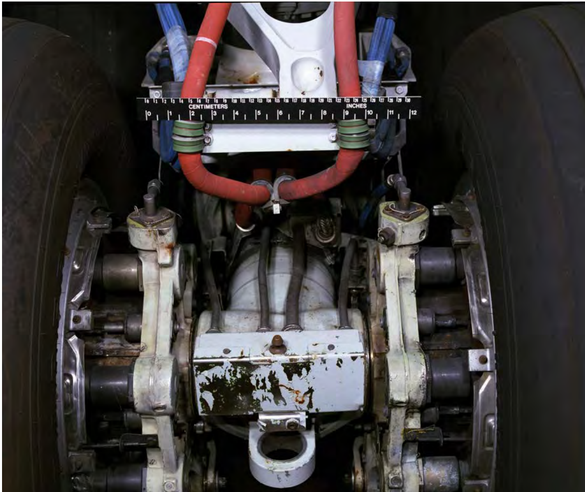
Figure 3-10. Main landing gear on the Boeing 757 was used in a landing gear noise study at NASA Langley Research Center in 1996 (NASA-LaRC photo EL-1996-00264).
