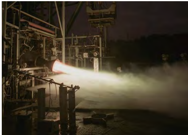
Figure 3-55. This photo shows an X-34 40K Fastrac II duration test performed at Marshall Space Flight Center in June 1997 (NASA-MSFC photo MSFC-9705975).
