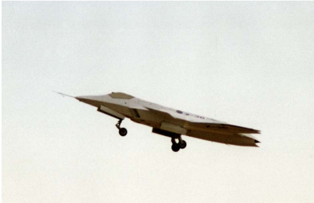
Figure 3-26. The remotely piloted X-36 Tailless Fighter Agility Research Aircraft lifts off on its first flight from Rogers Dry Lake at the Dryden Flight Research Facility on 17 May 1997. The aircraft flew for 5 minutes and reached an altitude of approximately 4,900 feet (1,493 meters) (NASA photo EC97-44064-3, by Carla Thomas).
