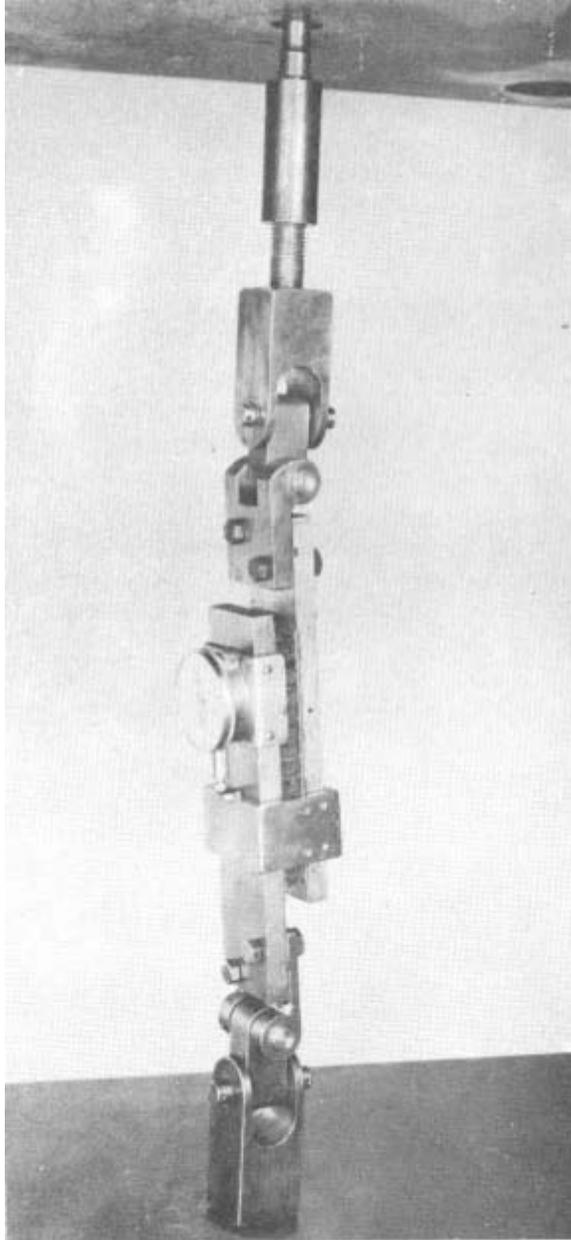
**Figure 4. --Apparatus for conducting shear tests of specimens cut from the test panels.**
