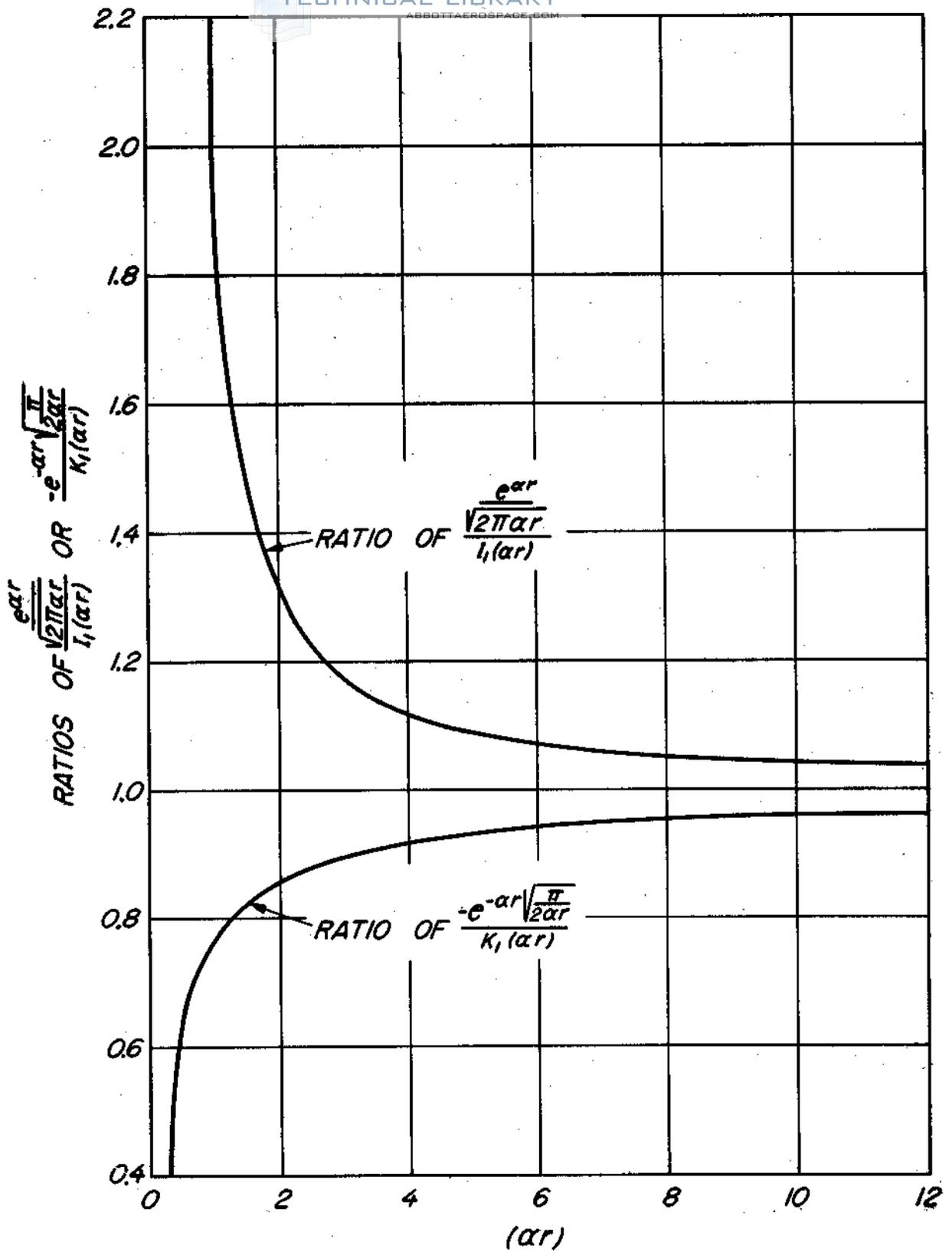
Figure 5. --Relationship between exponential functions and modified Bessel functions.
