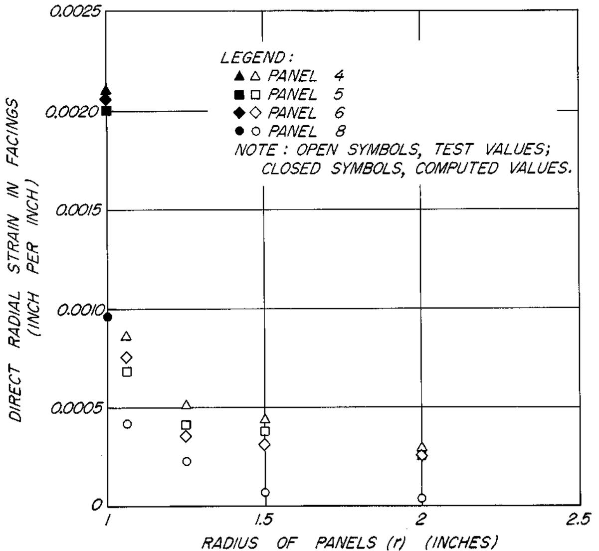
Figure 9.--Relationship between computed radial facing strains at edge of insert and observed facing strains near the insert. All panels had aluminum faces. Panels 4, 5, and 6 had balsa cores; panel 8 had a cork core.
