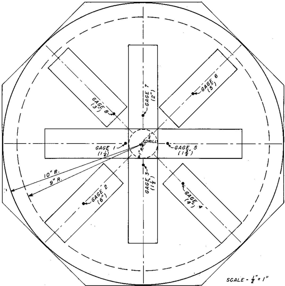
Figure 1. --Details of panel construction, locations of SR-4 gages in core, and the cutting pattern used to obtain shear specimens after the panels were tested.
