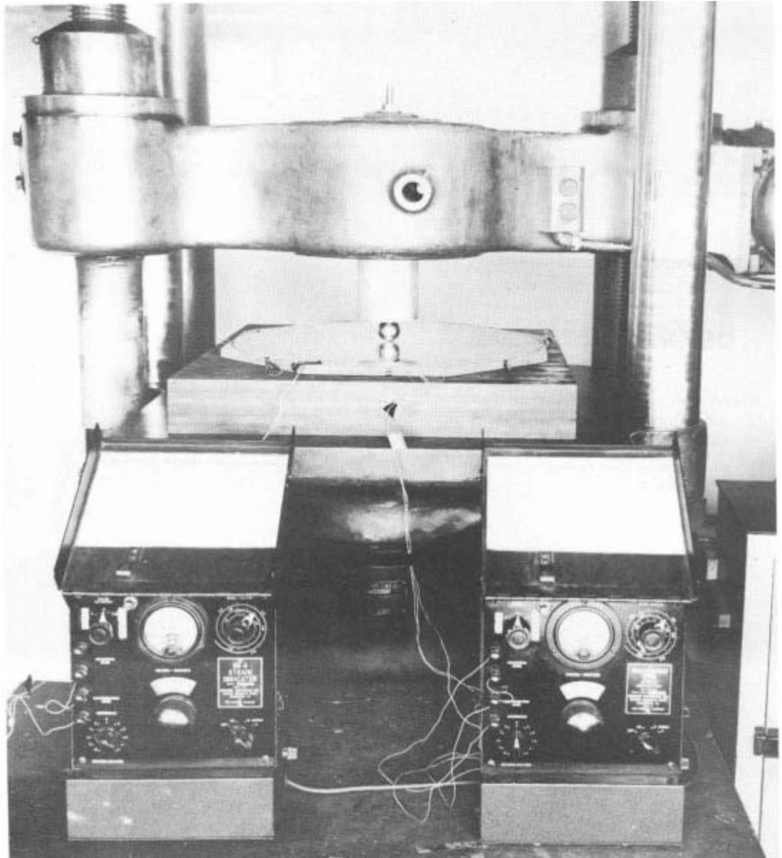
**Figure 3. --Cork core panel under test. Load was applied through a steel ball bearing to insure concentric loading of the insert. Two sets of gages were read at one time, and the test was repeated until all gages had been read.**
