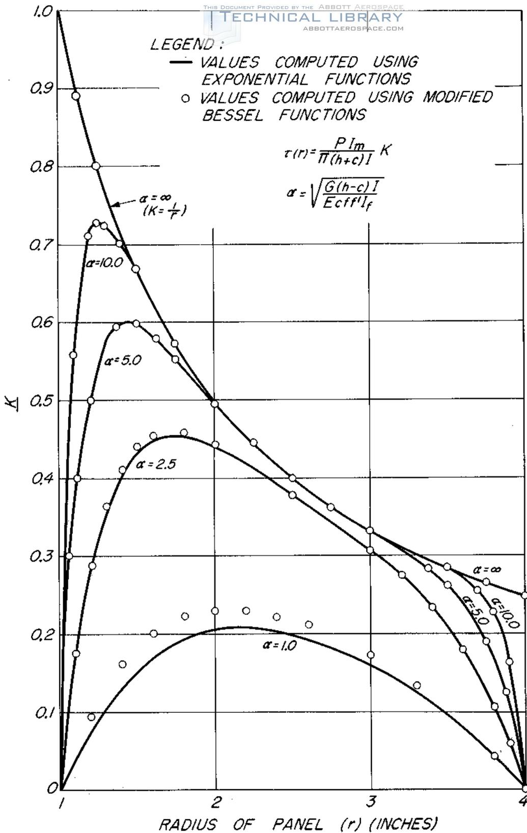
Figure 6. --Radial variation in shear stress in the core of a sandwich panel 8 inches in diameter with a central insert 2 inches in diameter.
