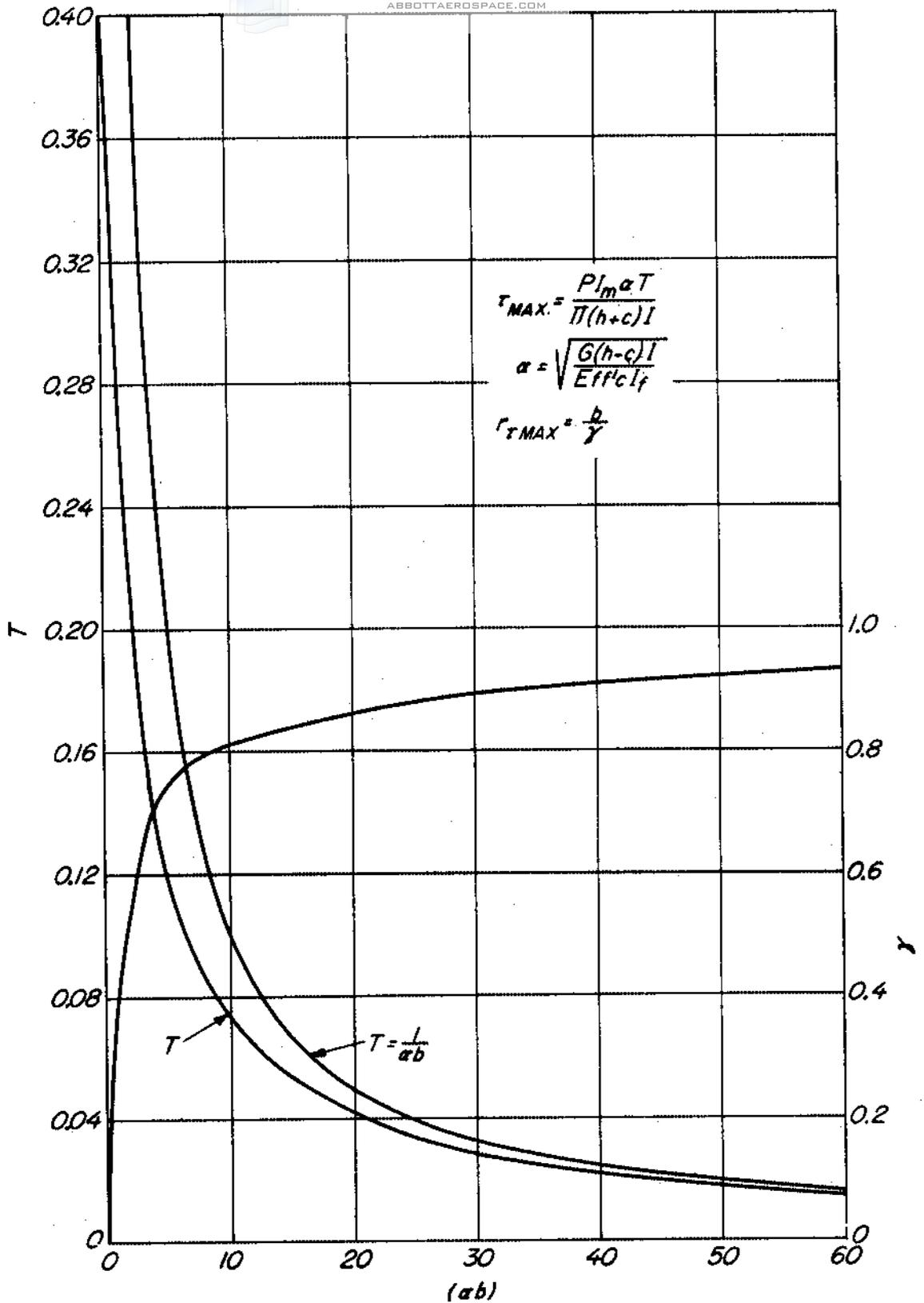
Figure 7.--Maximum shear stress in the core and its radial position for a large, circular sandwich panel with a small, normally loaded, circular insert.
