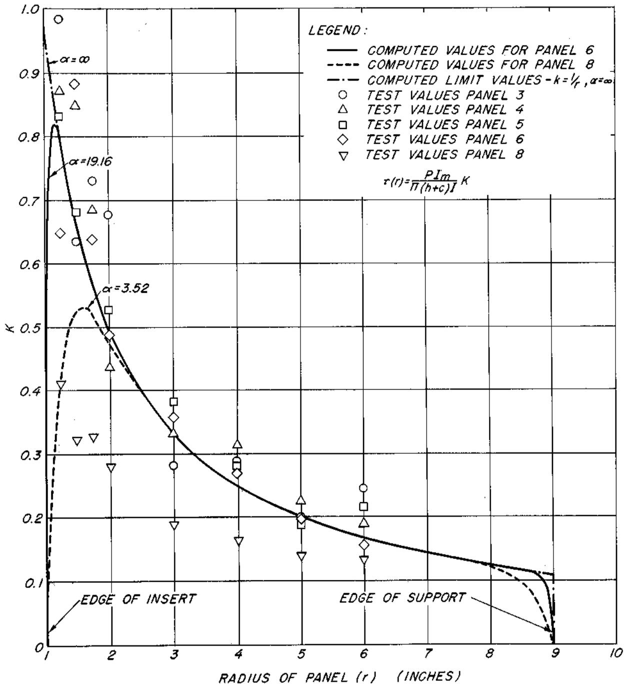
Figure 8.—Computed and observed radial variation in shear stress in the cores. Panels 3, 4, 5, and 6 had balsa cores and aluminum faces; panel 8 had a cork core and aluminum faces.
