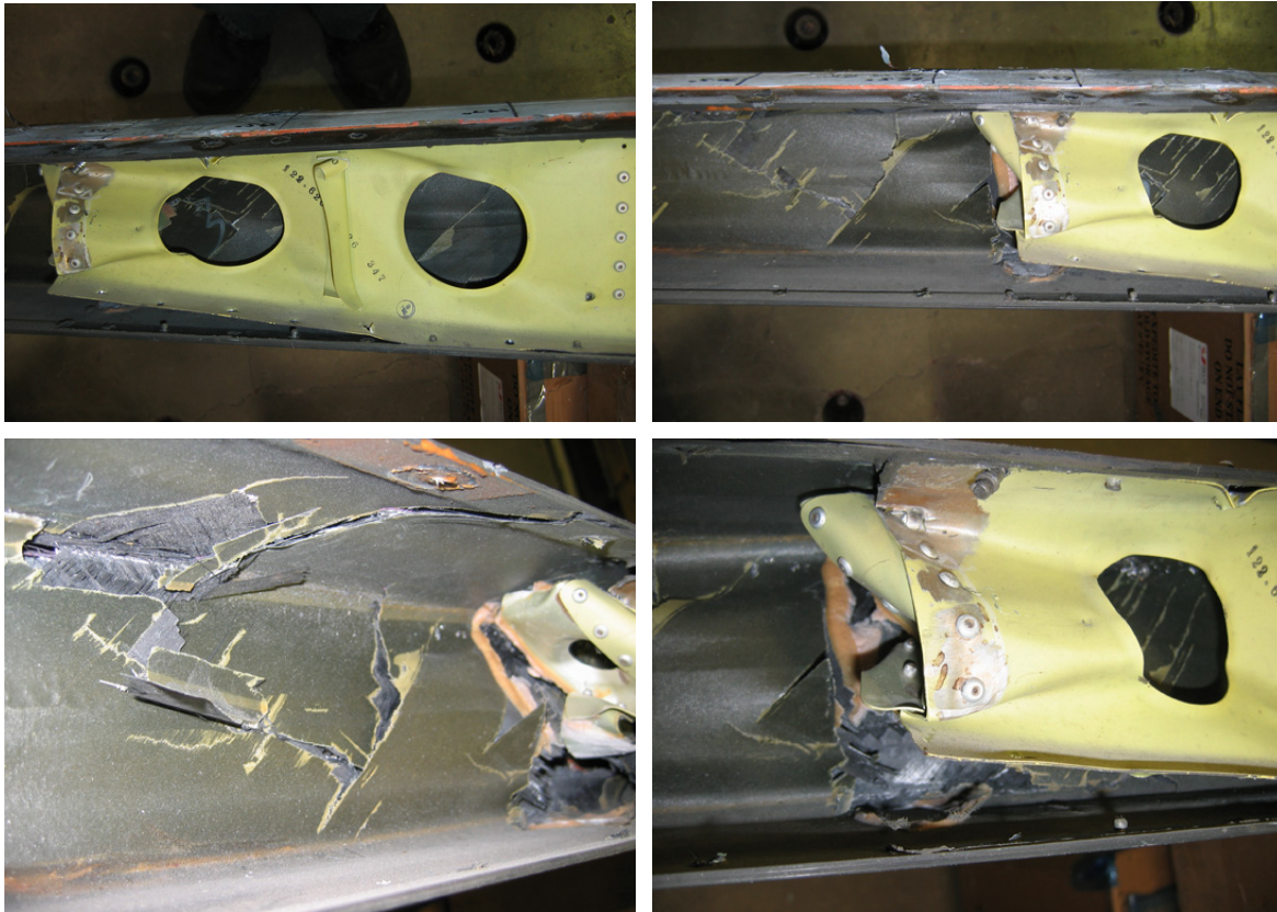
Figure 134. Post-test inspections of ST003 upon removal of leading edge.
