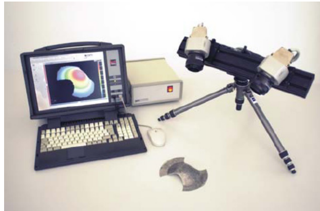
Figure 8. Portable version of ARAMIS photogrammetry system [51].
