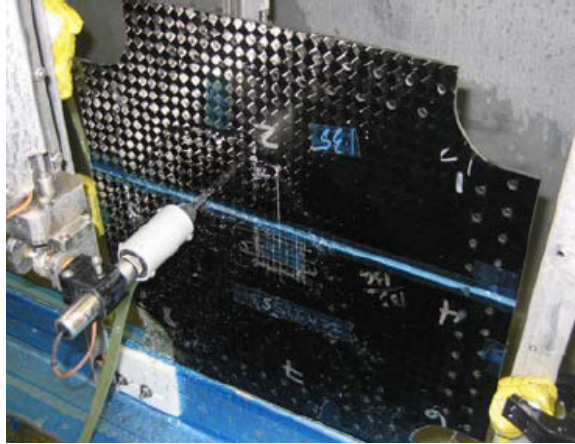
Figure 7. TTU scanning of PFS test specimen.
