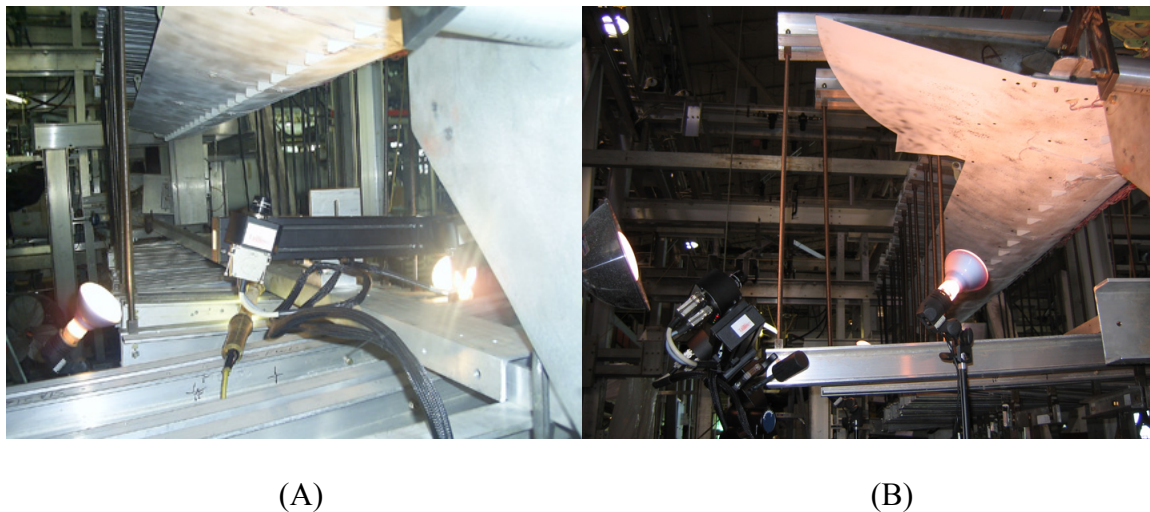
Figure D.2. ARAMIS System setup (a) up to, and (b) after the limit load.
