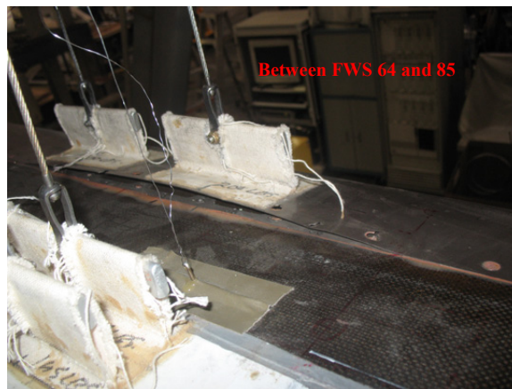
Figure 128. Leading-edge fastener pullout failure (bottom surface) after 2.0 DLT.
