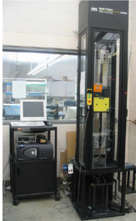
Figure 5. Instron Dynatup drop-weight tester.
