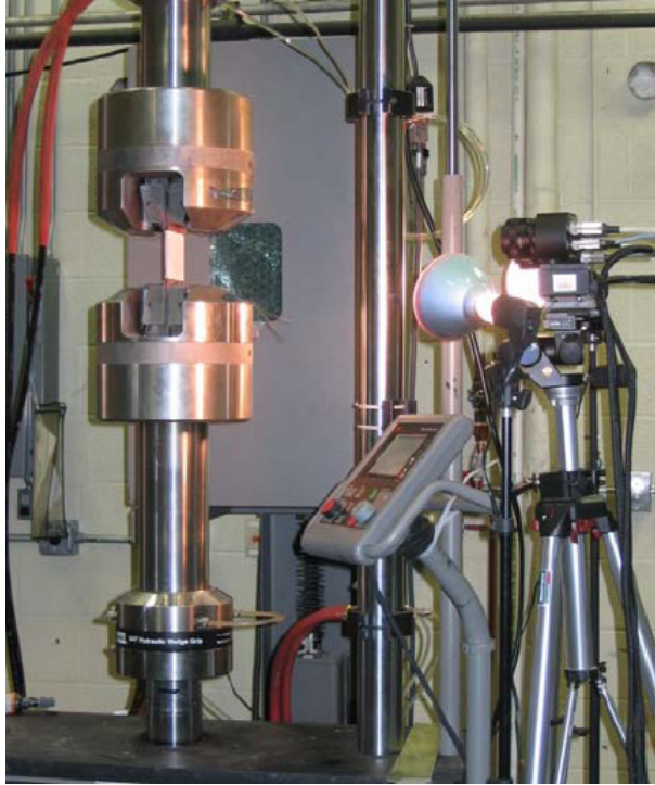
Figure 10. MTS servo-hydraulic test frame.
