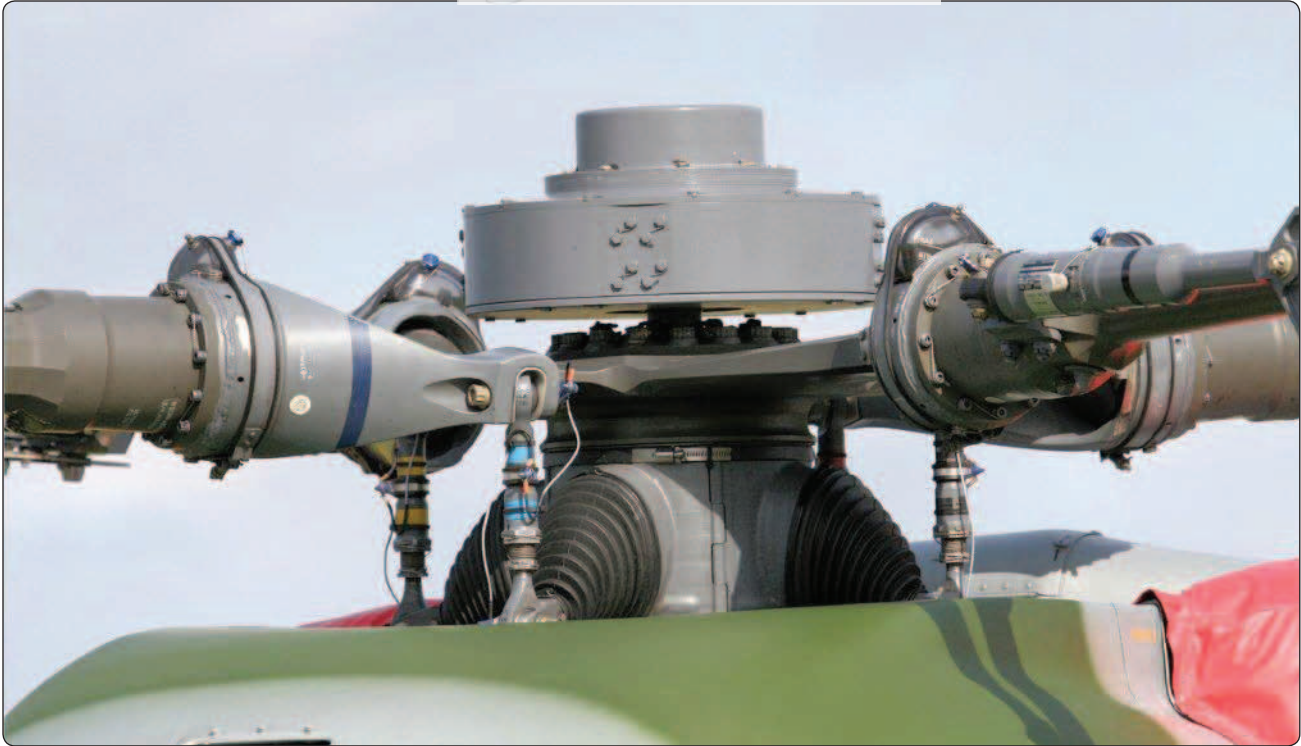
Figure 5-3. A Westland Lynx four-blade rigid main rotor.
