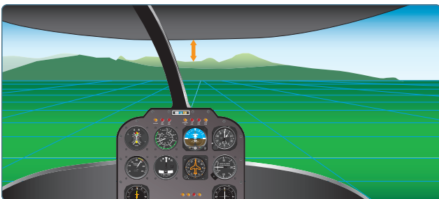
Figure 10-1. Maintain a straight-and-level altitude by keeping the tip-path plane parallel to and a constant distance above or below the natural horizon.
