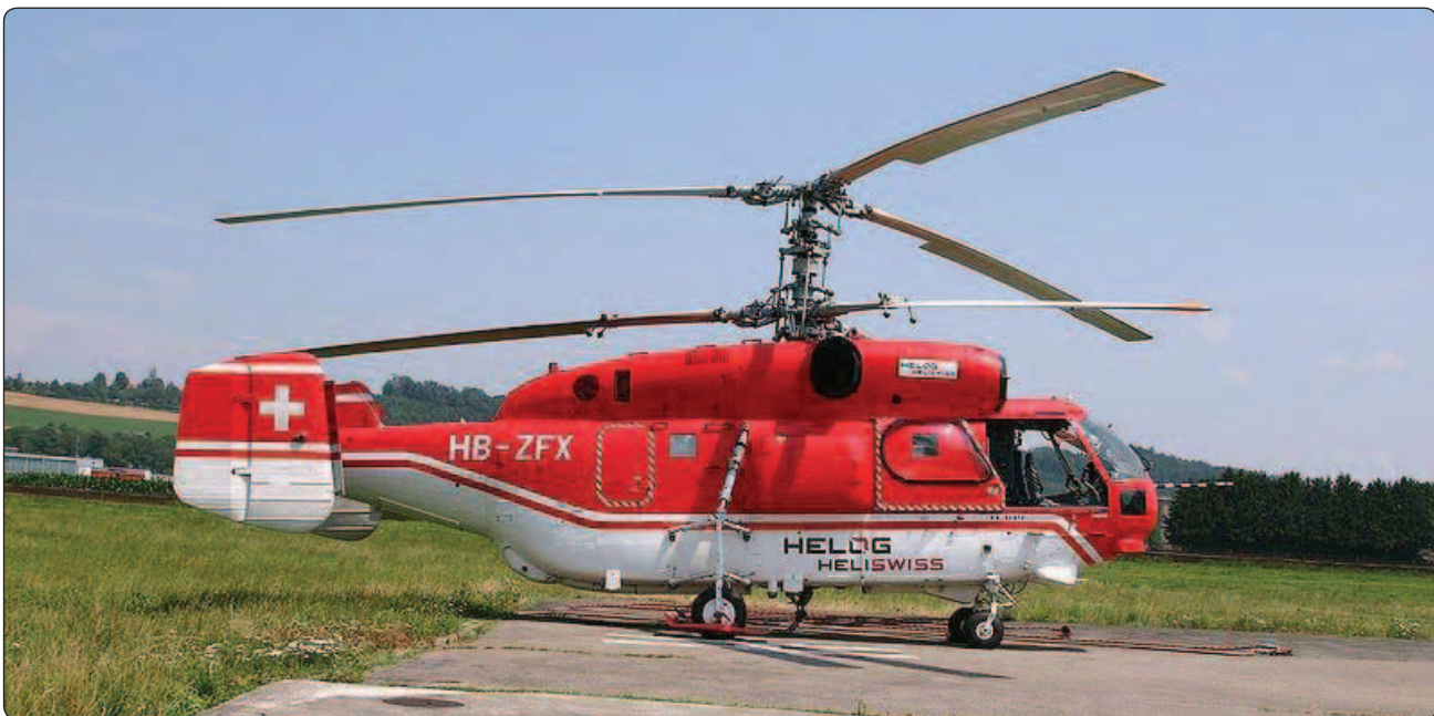
Figure 5-15. A Kamov Ka-32A-12 has a coaxial rotor system.
