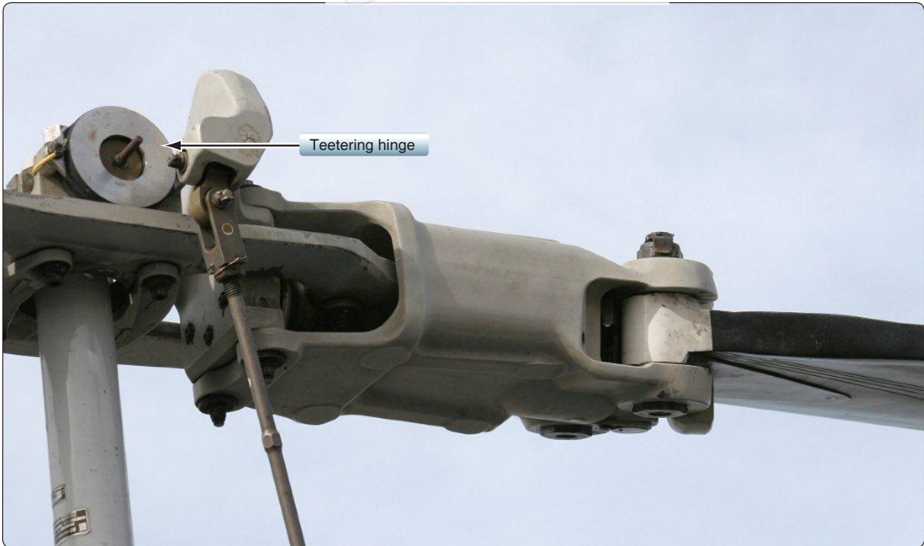
Figure 5-7. Main rotor blade grip of the Bell 230 semirigid rotor system.
