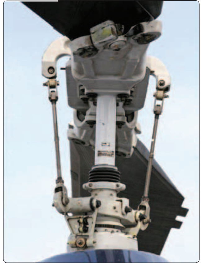
Figure 5-5. Bell 230 semirigid rotor system and swashplate assembly.
