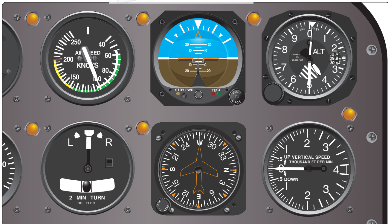
Figure 13-1. Instruments that should be discussed when teaching instrument flying: airspeed indicator, attitude indicator, altimeter, turn indicator, heading indicator, and vertical speed indicator (VSI).
