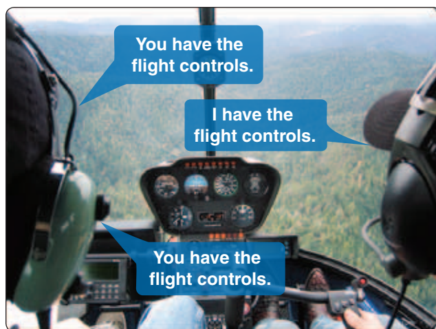
Figure 9-3. Exchanging flight controls.
