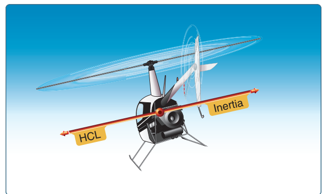
Figure 10-2. During a level, coordinated turn, the rate of turn is commensurate with the angle of bank used, and inertia and horizontal component of lift (HCL) are equal.
