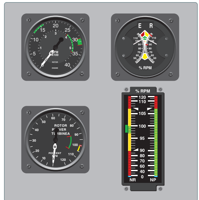
Figure 5-25. There are various types of dual-needle tachometers; however, when the needles are superimposed or joined, the engine rpm ratio is the same as the gear reduction ratio.
