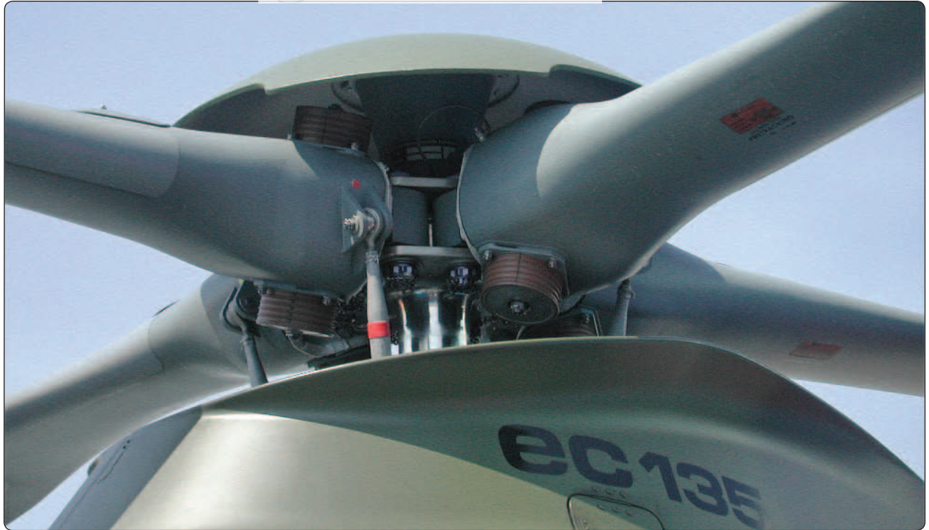
Figure 5-12. A Eurocopter EC-135 hingeless and bearingless rotor.
