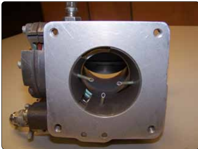
Figure 2-32. Impact tubes for inlet air pressure.
