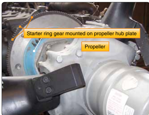
Figure 5-10. Starter ring gear mounted on the propeller hub.
