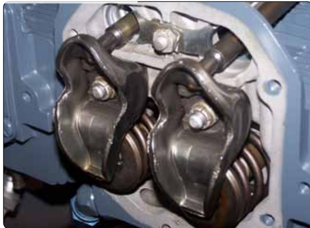
Figure 1-31. Rocker opposed engine arms.
