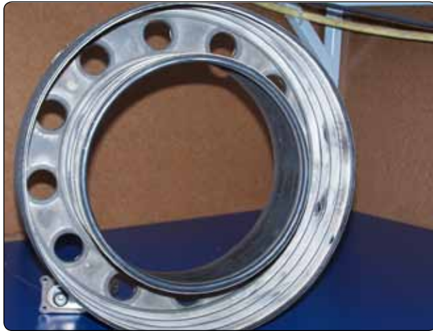
Figure 1-58. Annular combustion with chamber ceramic coating.
