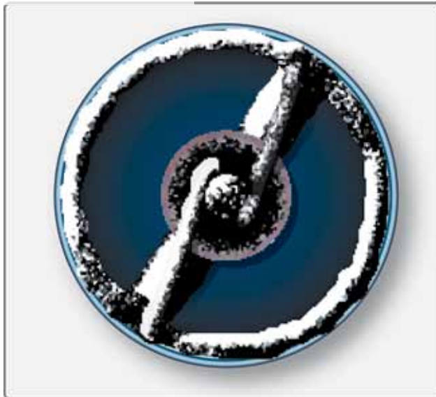
Figure 4-48. Carbon fouled spark plug.
