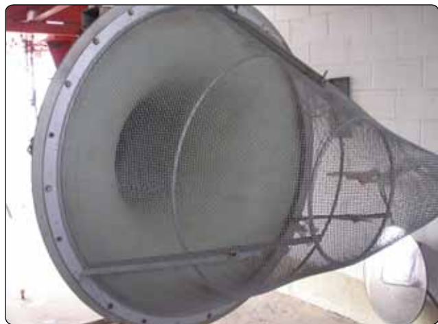
Figure 3-30. A bellmouth inlet used during system tests.
