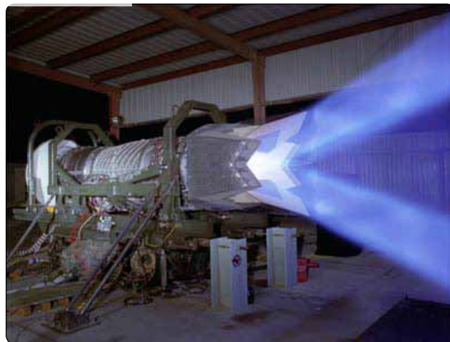
Figure 3-51. A pilot can direct thrust via the vectoring nozzle 20° up or down to increase flight maneuverability.
