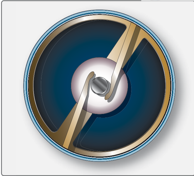
Figure 4-50. Spark plug gap erosion.
