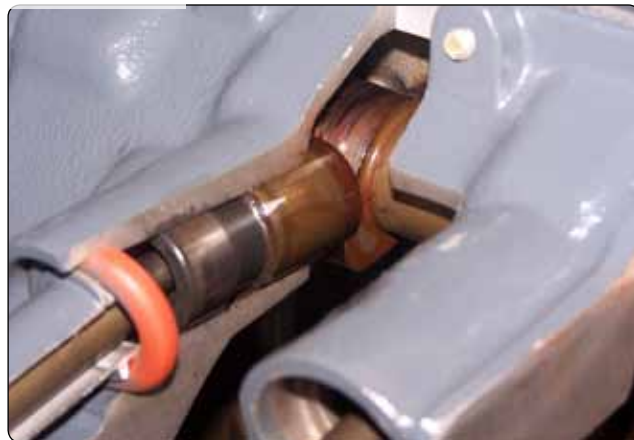
Figure 1-29. Cam load on lifter body.
