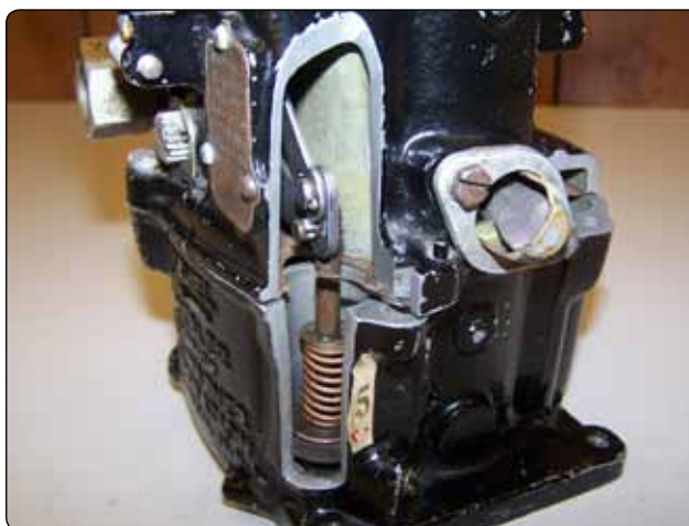
Figure 2-19. Accelerating pump shown in cutaway.
