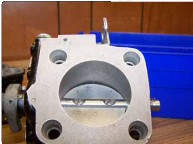
Figure 2-14. Throttle action in idle position.
