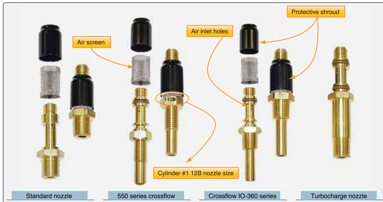
Figure 2-45. Fuel discharge nozzles.
