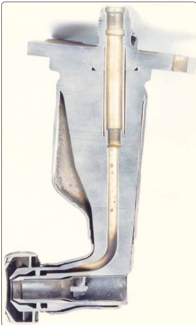
Figure 2-64. Simplex airblast nozzle cutaway.
