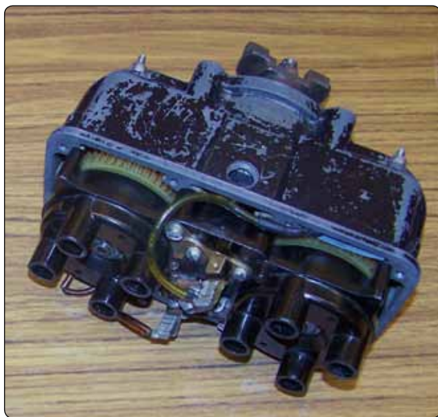
Figure 4-18. A dual magneto with two distributors.
