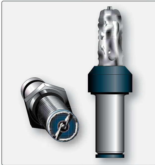
Figure 4-49. Lead fouled spark plug.
