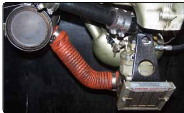
Figure 3-5. Location of a carburetor heat air valve.
