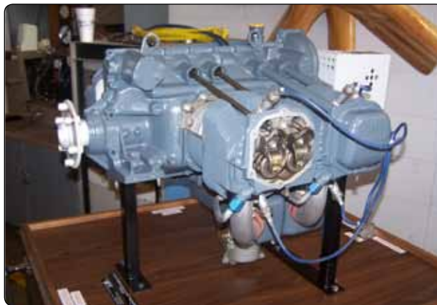
Figure 1-1. A typical four-cylinder opposed engine.
