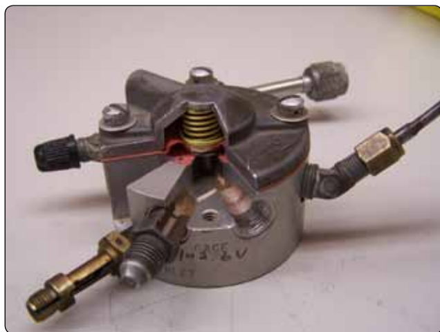
Figure 2-37. Flow divider cutaway.
