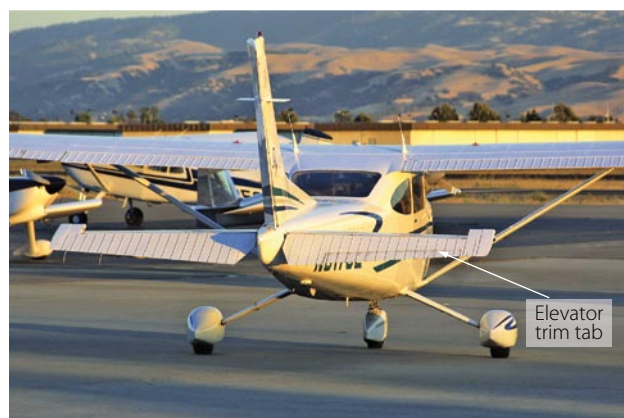
Figure 3-71. Elevator trim tab on a Cessna 182.
