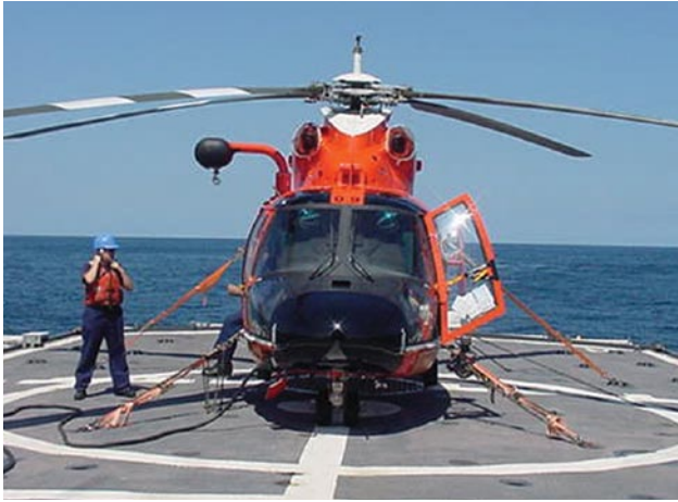
Figure 11-13. Example of mooring of a helicopter.
