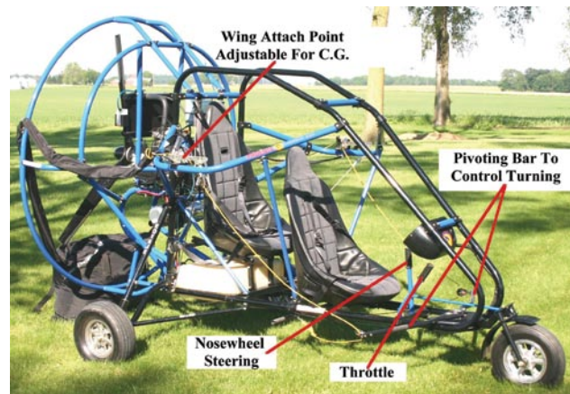
Figure 4-39. Powered parachute structure with wing attach points.
