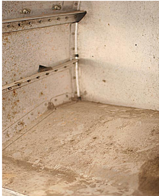
Figure 6-2. Direct chemical attack in a battery compartment.
