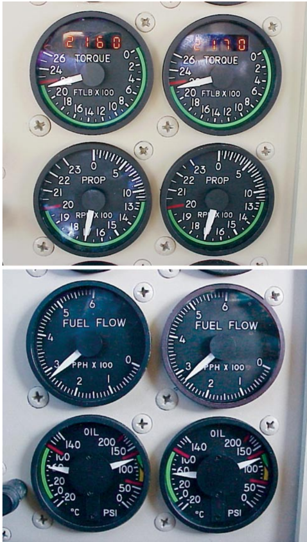
Figure 11-15. Typical examples of turboprop instruments.
