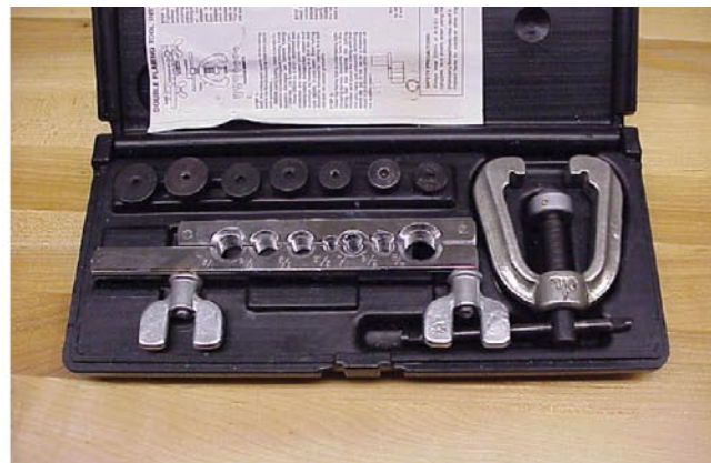
Figure 7-10. Double flare tool.
