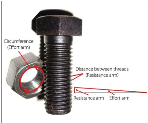
Figure 3-18. A bolt and nut as an inclined plane.
