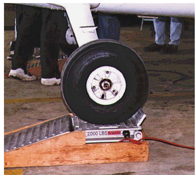
Figure 3-17. Ramp in use with a Cessna 172.
