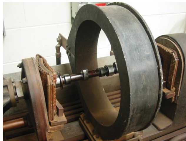
Figure 8-17. Longitudinal magnetization of crankshaft (solenoid method).
