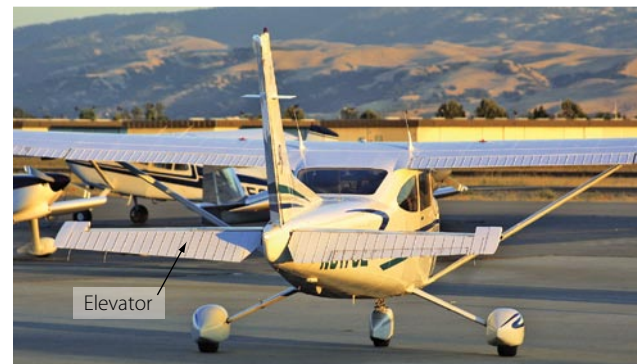
Figure 3-65. Elevator on a Cessna 182 provides pitch control.
