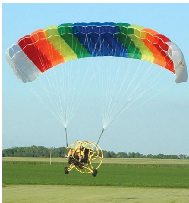
Figure 3-102. Powered parachute with the wing inflated.
