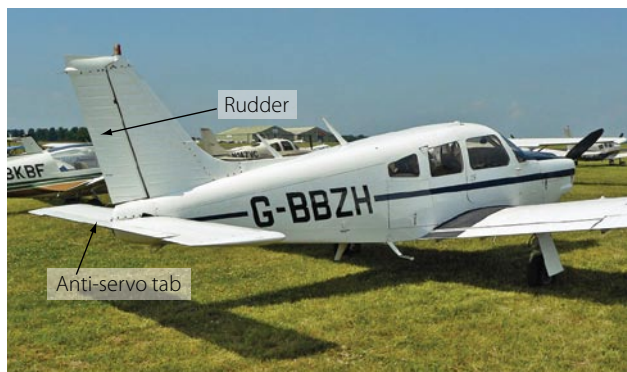
Figure 3-70. Rudder on a Piper Cherokee Arrow.
