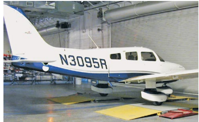
Figure 4-12. Weighing a Piper Archer using electronic platform scales.
