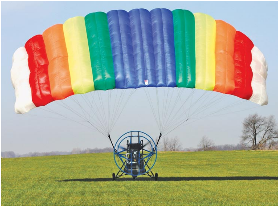
Figure 3-104. Powered parachute wing trailing edge.
