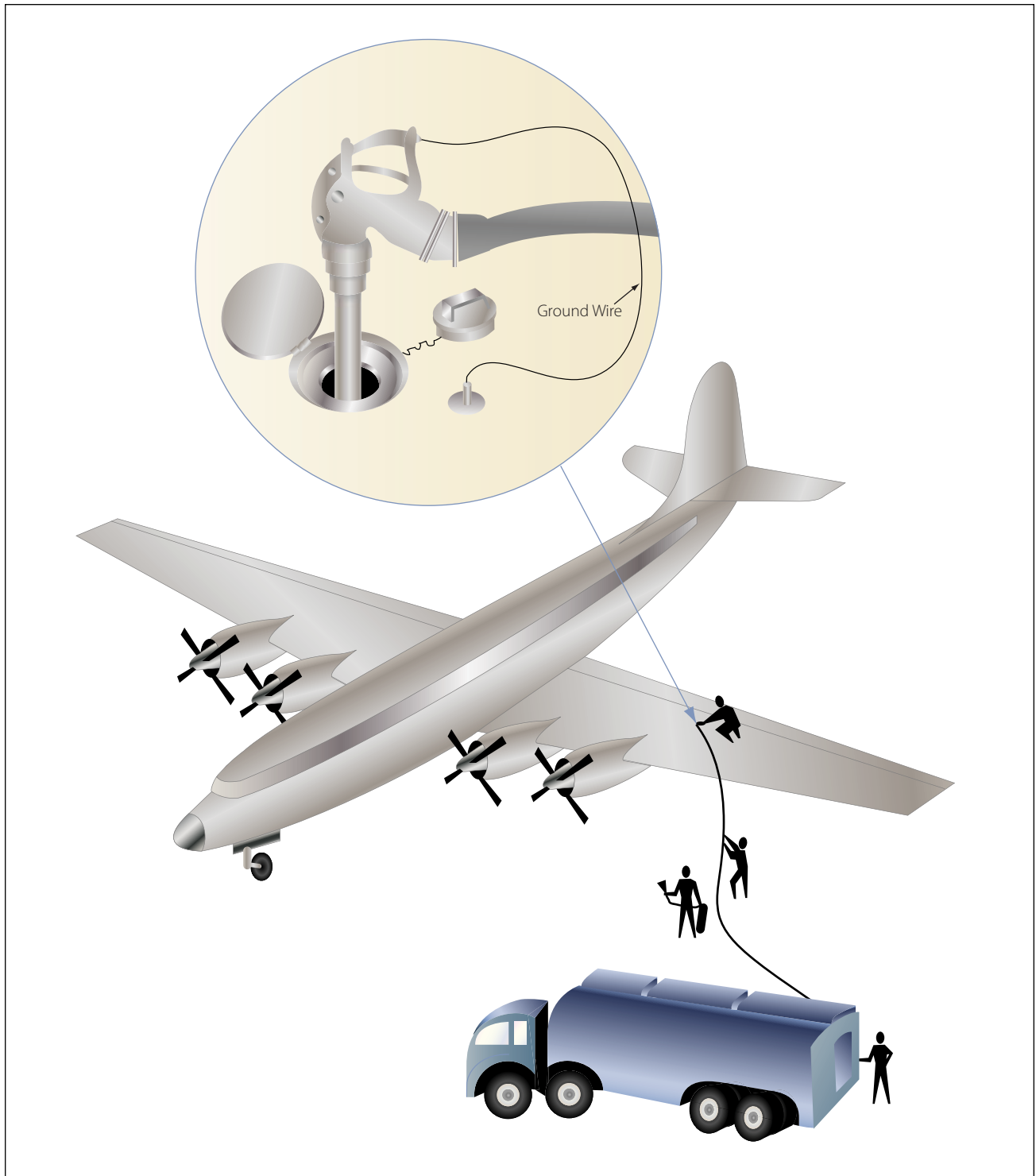
Figure 11-31. Refueling an aircraft by the over-the-wing method.
