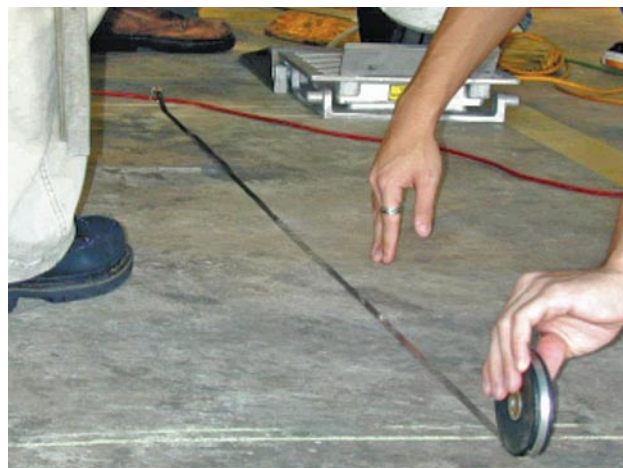
Figure 4-18. Measuring the nosewheel arm on a Cessna 310.
