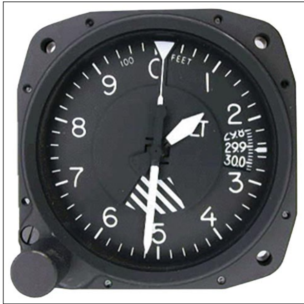
Figure 3-51. An airplane's altimeter is an aneroid barometer.
