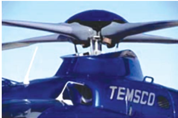
Figure 3-85. Eurocopter Model 135 rigid rotor system.
