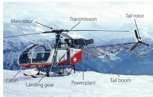
Figure 3-81. Main components of a helicopter.
