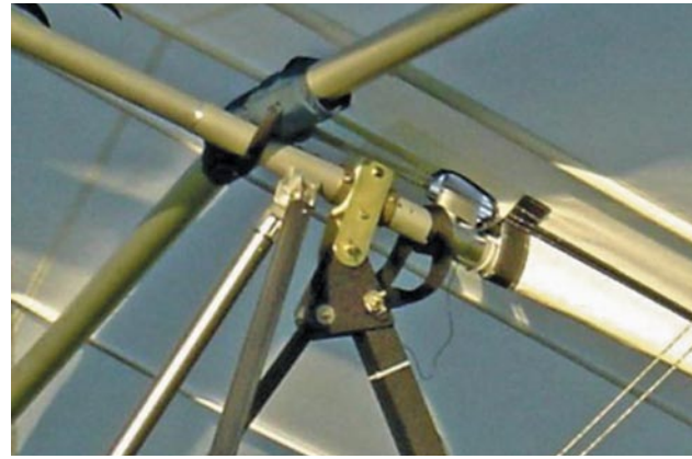
Figure 4-38. Wing attach point for a weight-shift aircraft.
