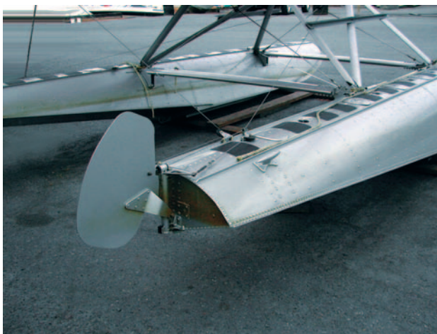
Figure 4-4. Inspect the water rudders, cables, springs, and pulleys for proper operation.
