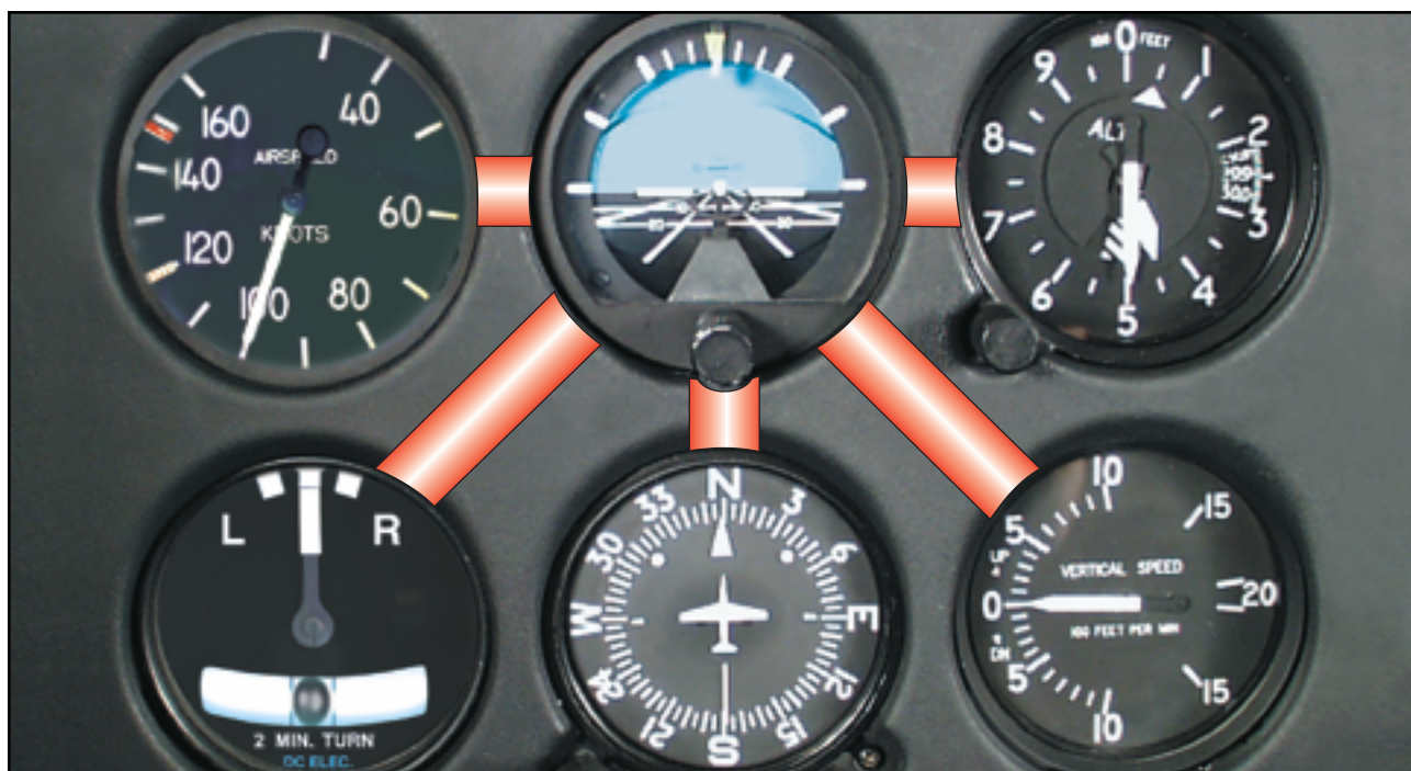
Figure 12-10. In most situations, the cross-check pattern includes the attitude indicator between the cross-check of each of the other instruments. A typical cross-check might progress as follows: attitude indicator, altimeter, attitude indicator, VSI, attitude indicator, heading indicator, attitude indicator, and so on.
