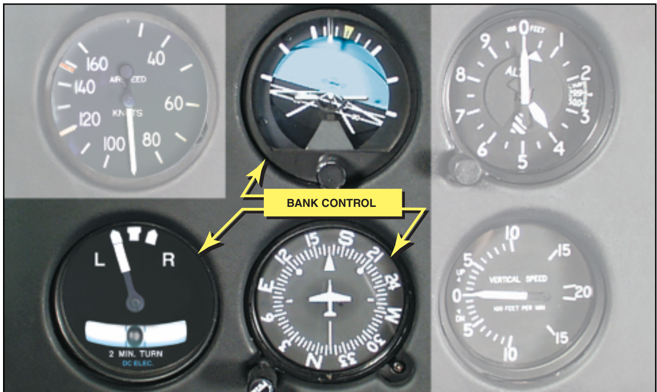
Figure 12-13. The flight instruments used for bank control are the attitude, heading, and turn indicators.
