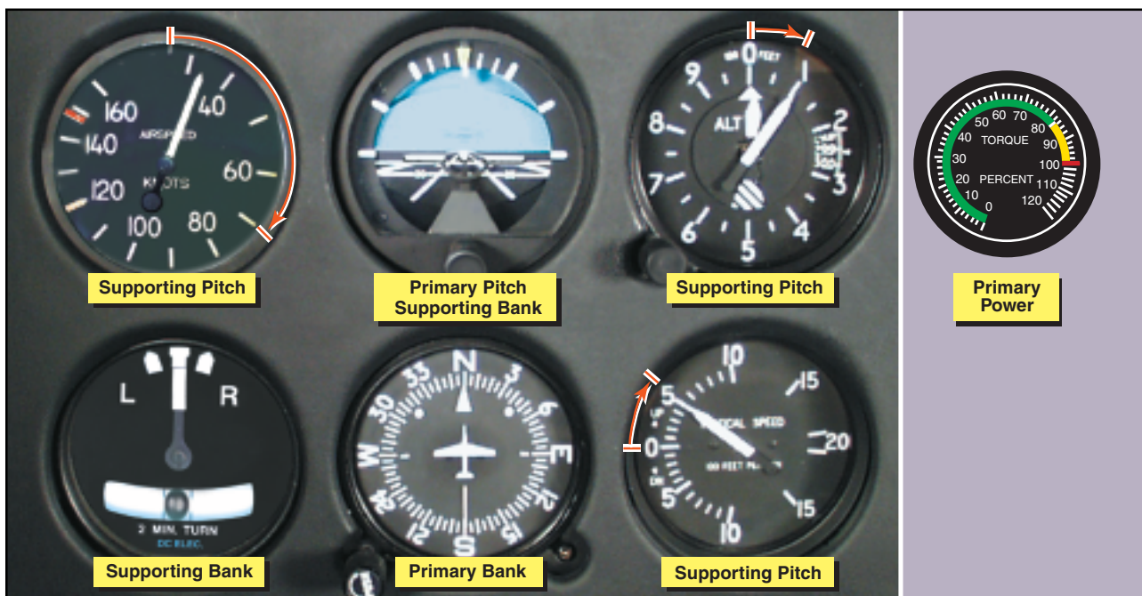
Figure 12-22. Flight instrument indications during an instrument takeoff.
