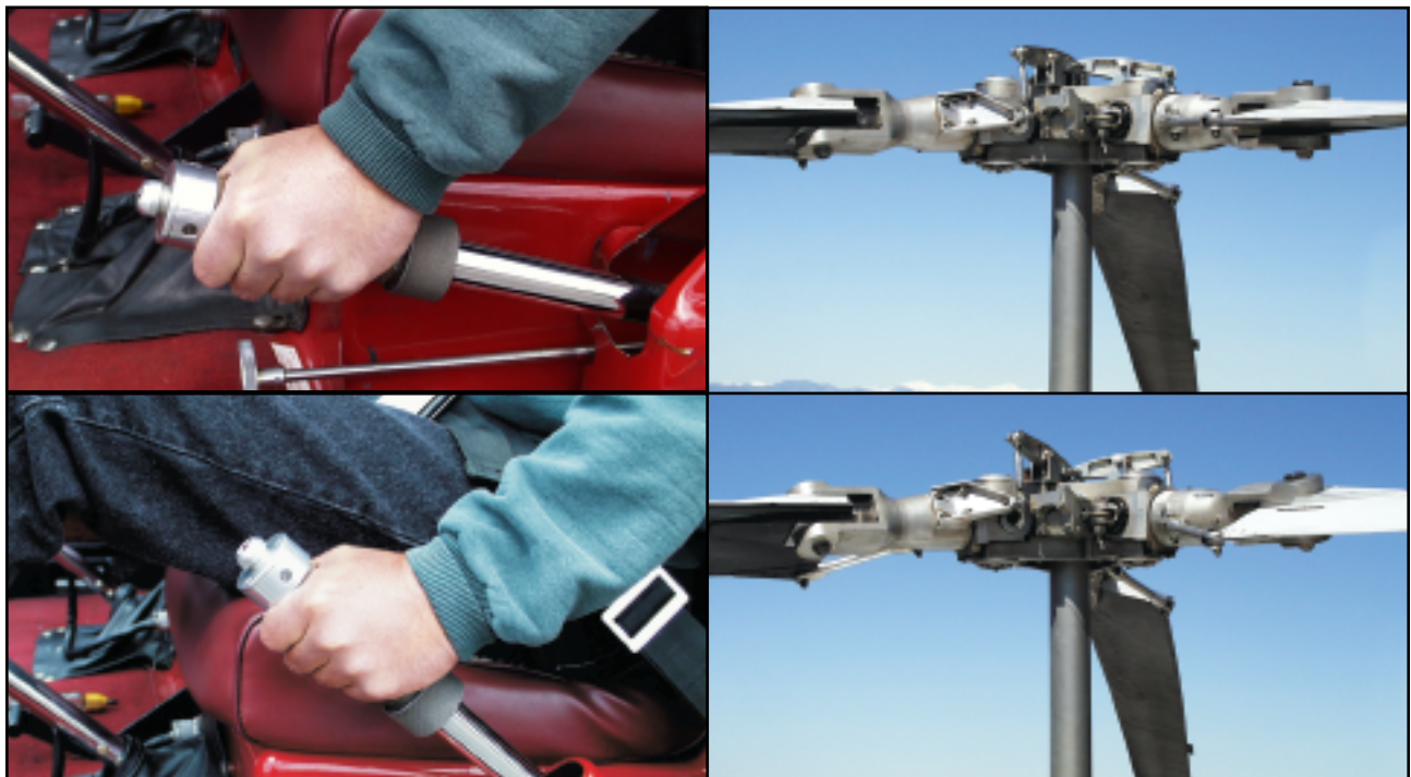
Figure 4-1. Raising the collective pitch control increases the pitch angle the same amount on all blades.
