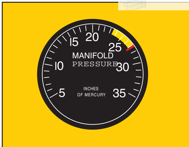
Figure 6-5. A manifold pressure gauge is commonly used with piston-powered aircraft.
