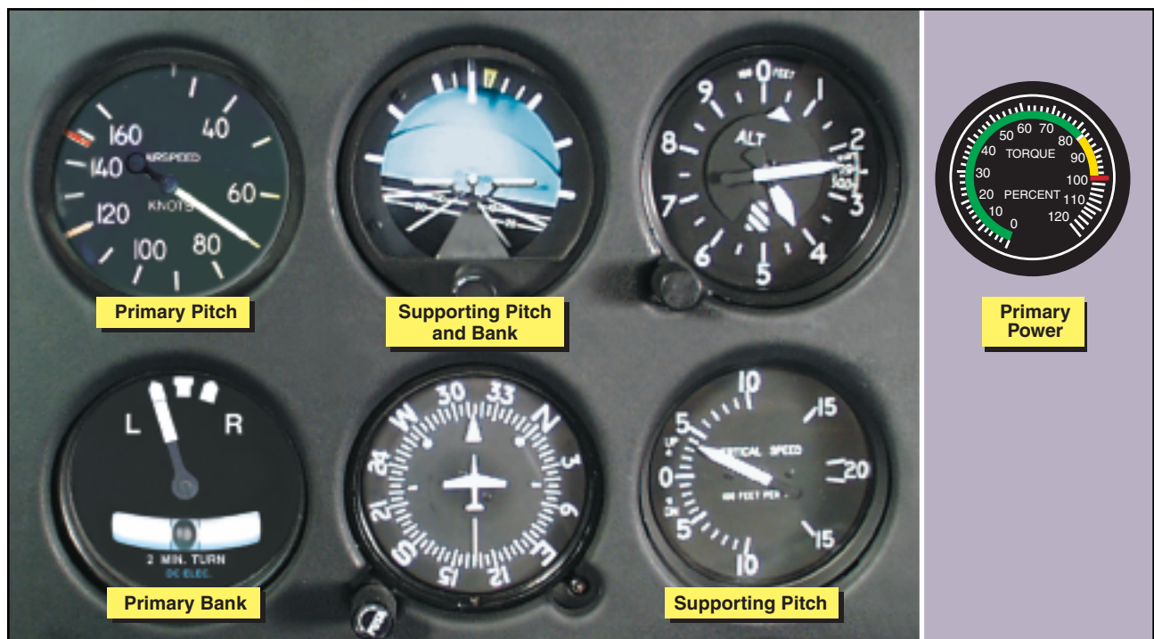
Figure 12-21. Flight instrument indications for a stabilized left climbing turn at a constant airspeed.
