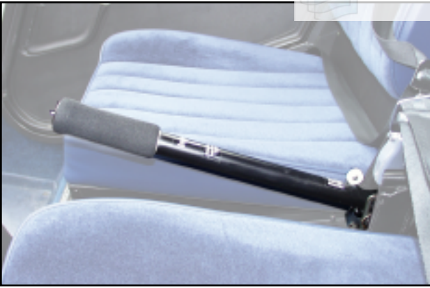
Figure 4-2. A twist grip throttle is usually mounted on the end of the collective lever. Some turbine helicopters have the throttles mounted on the overhead panel or on the floor in the cockpit.
