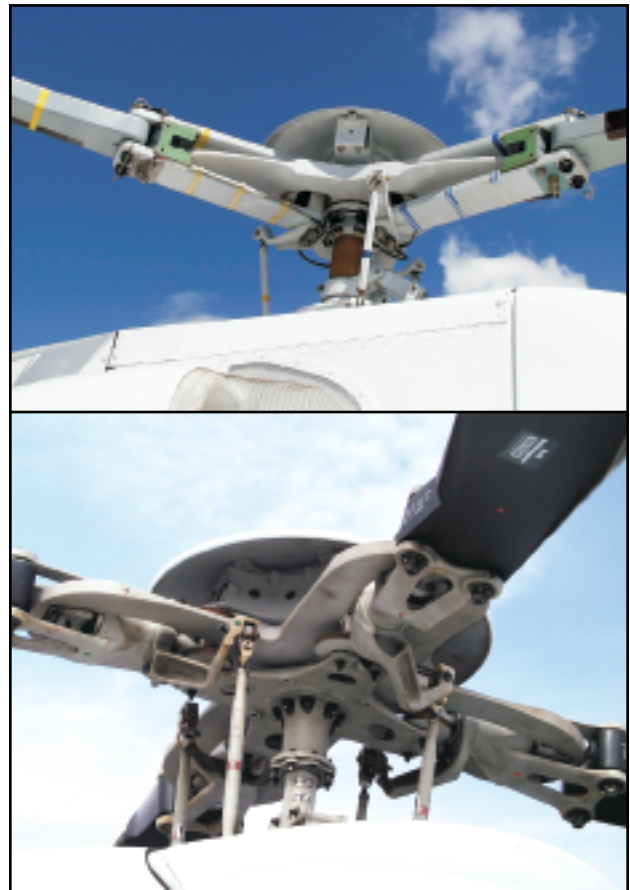
Figure 5-7. Rotor systems, such as Eurocopter's Starflex or Bell's soft-in-plane, use composite material and elastomeric bearings to reduce complexity and maintenance and, thereby, increase reliability.
