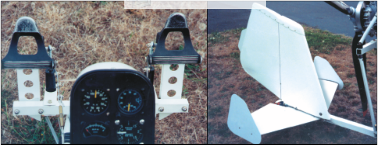
Figure 17-3. Foot pedals provide rudder control and operation is similar to that of an airplane.
