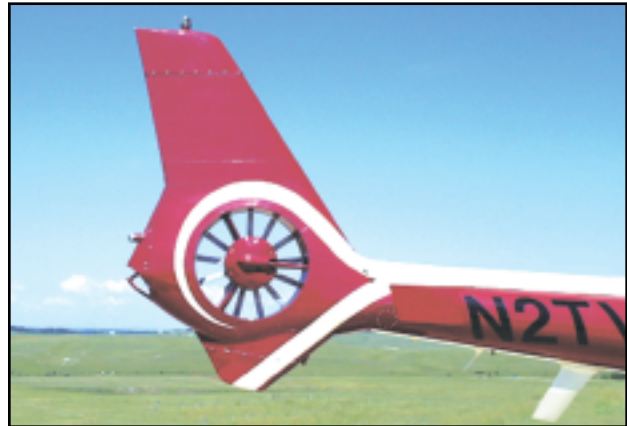
Figure 1-4. Compared to an unprotected tail rotor, the fenestron antitorque system provides an improved margin of safety during ground operations.
