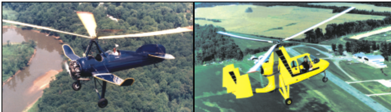
Figure 15-1. The gyroplane may have wings, be either tractor or pusher configured, and could be turbine or propeller powered. Pictured are the Pitcairn PCA-2 Autogyro (left) and the Air & Space 18A gyroplane.
