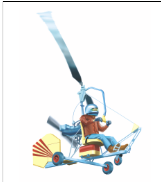
Figure 17-2. The direct overhead stick attachment has been used for control of the rotor disc on some gyroplanes.
