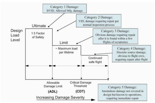
Figure 3 - Schematic diagram of design load levels versus categories of damage severity
