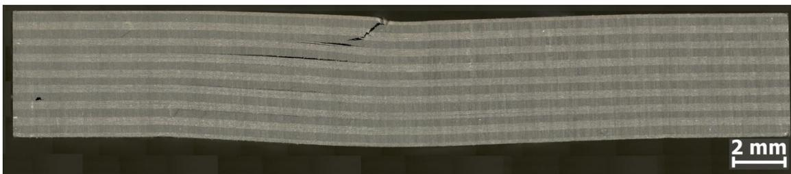
Figure 54. Panel 8 failed H/W SBS specimen from center.
