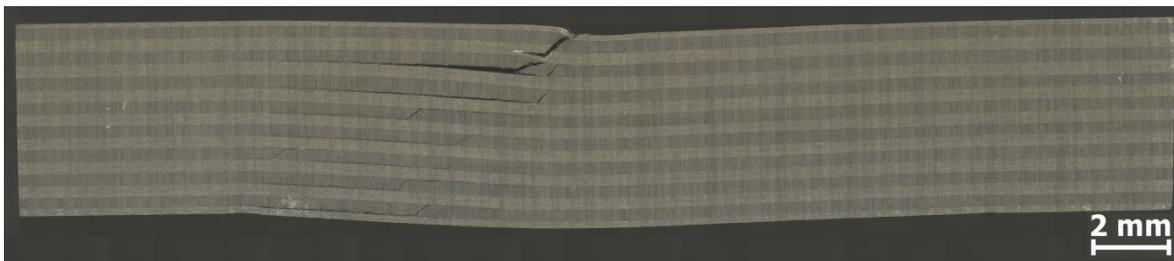
Figure 53. Panel 7 failed H/W SBS specimen from center.
