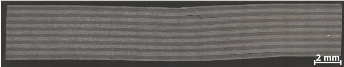
Figure 48. Typical failed H/W SBS specimen of panels 1 to 4.
