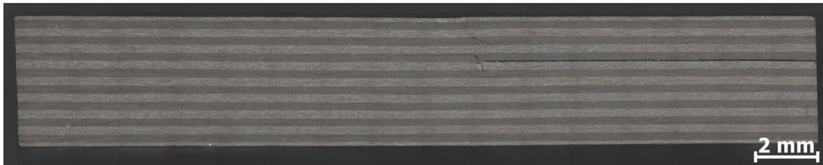
Figure 36. Typical failed RT/D SBS specimen of panels 1 to 5.
