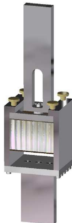
Figure 27-1: Manufacture control: Out-of-plane test fixture for tension (pull-out) tests
