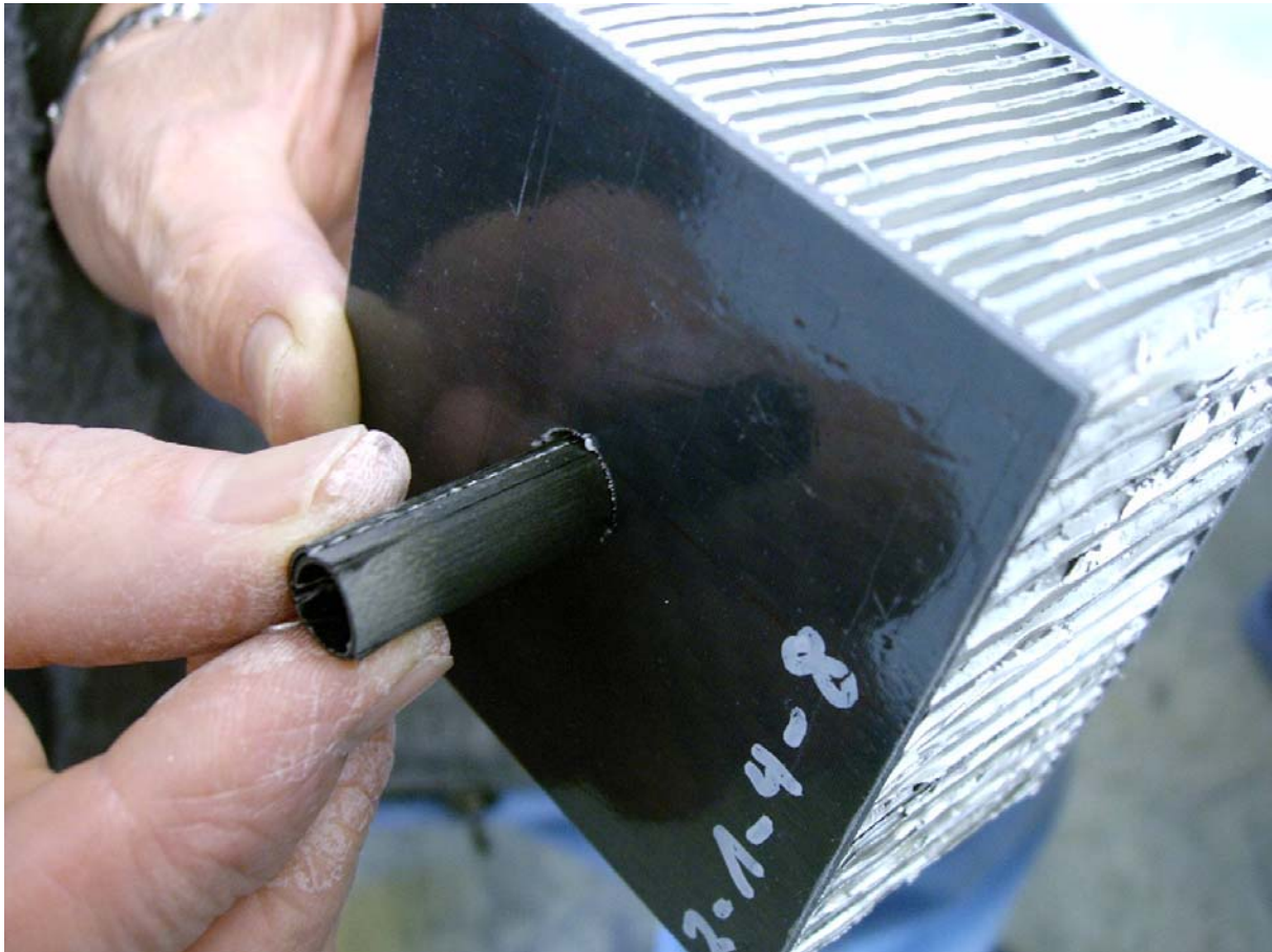
Figure A-2: Carbon fibre tube inserts: Fitting of spreadable CFRP tube
