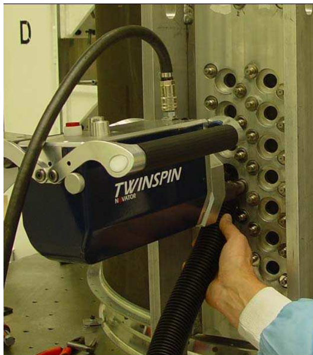
Figure 39.10-2 – Orbital drilling: Equipment mounted on a jig
