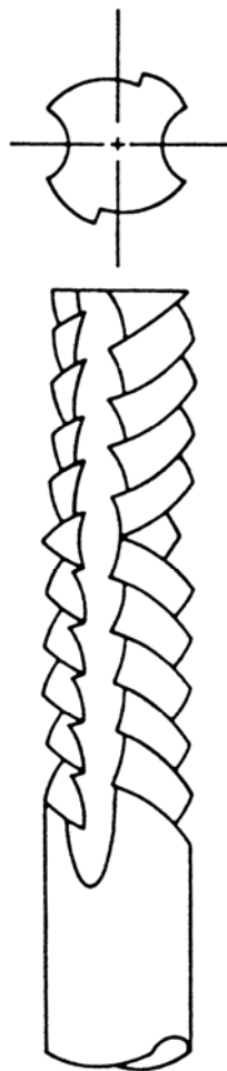
Figure 39.3-1 - Router: Opposed helix for aramid/epoxy
