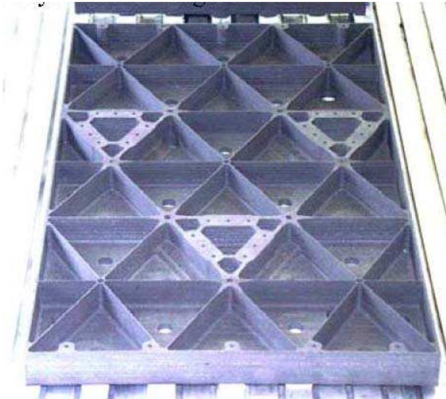
Figure 43.12-4 – Cestic® ceramic: Example of integrally-stiffened panel
