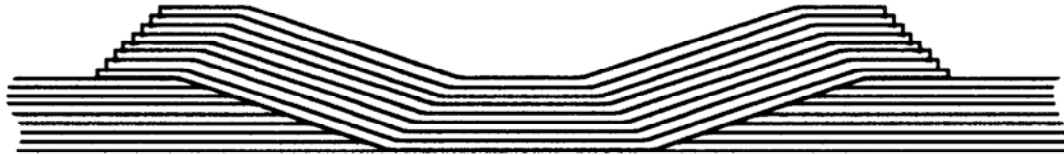
Figure 41.5-2 - Flush repair, used by Airbus Industrie
