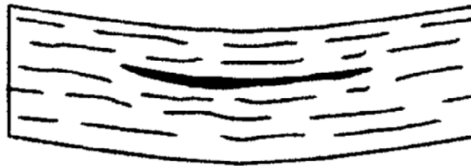
Figure 41.3-5 - Damage categories: Delamination
