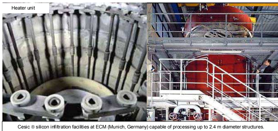
Figure 43.12-2 – Cesic®: Silicon-infiltration processing equipment
