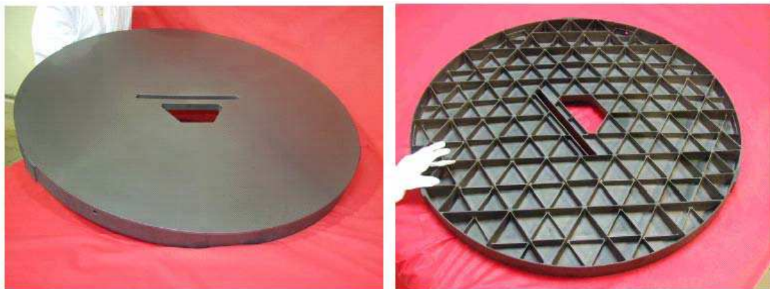
Figure 43.12-8 – SiC-100®: 1m diameter 'Demonstration Mirror' – ready to polish
