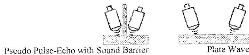
Figure 34.10-5 - Non-contact ultrasonics: Air-coupled sensor configurations
