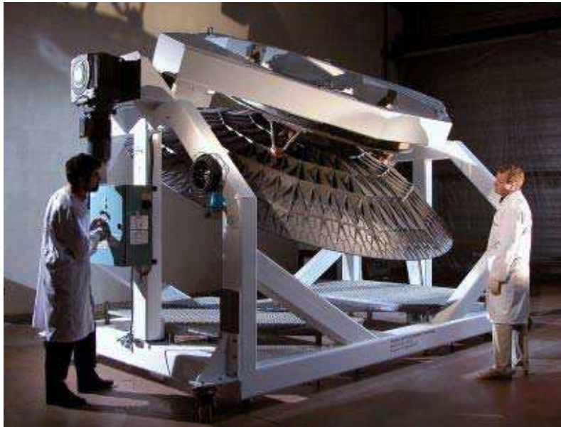
Figure 43.12-12 – SiC-100®: 3.5 m diameter HERSCHEL Primary Mirror – after assembly
