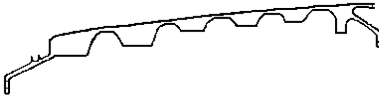
4.a - Ring Disk Drum Rotor Cross Section
